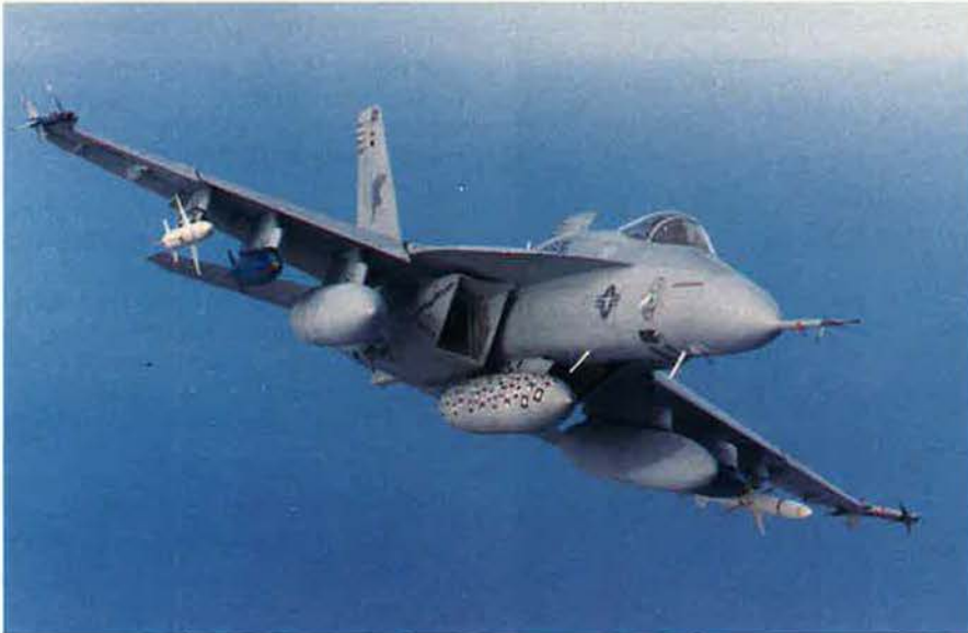
The heaviest Hornet: F/A-18E/F Super Hornet E1 took off carrying three 480-gallon fuel tanks, two Mk. 84 bombs, two AGM-88 High-Speed Antiradiation Missiles, and two AIM-9 Sidewinder missiles externally and flew without incident during tests at NAS Patuxent River, Md., in February.
