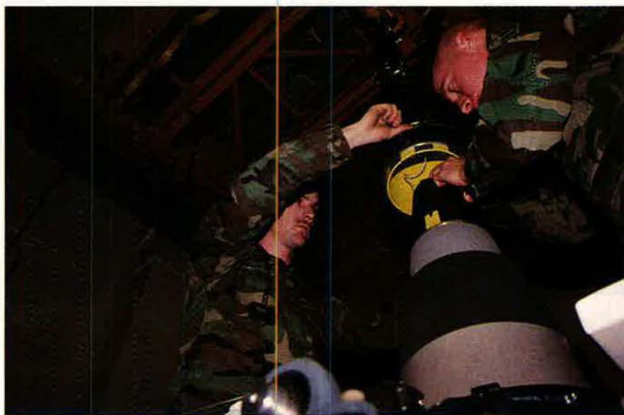
Like the rest of the missile, the reentry vehicles are periodically checked and maintained. At Ft. E. Warren, SSgt. Gary J. Skowronek, reentry vehicle maintenance team chief, goes by the book in overseeing the replacement of the last of up to 10 independently targetable reentry vehicles for the business end of an LGM-118A Peacekeeper missile. The Peacekeeper, fully operational since 1988, is larger, heavier, and more accurate than the Minuteman. The Styrofoam ring around one of the reentry vehicles protects it and also serves as a place for technicians to place their tools temporarily. At right, SrA. Kelly Summerfield and SrA. Mark Poani (right) carefully replace the cap on a reentry vehicle. Below, on the Minuteman III side of the base's weapons facility, SrA. Corey LaRack and SrA. James Cailari (right) check the forward component of the reentry system.
