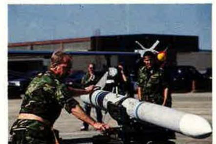
Above, a load crew prepares an AIM-120 Advanced Medium-Range Air-to-Air Missile for loading.
