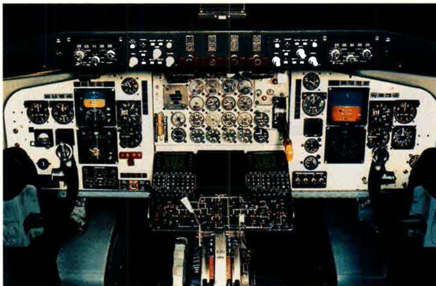
Rockwell International formally rolled out the first USAF C/KC-135 Pacer Crag July 19 with major avionics upgrades for the thirty-year-old aircraft. They include an FMS-800 Flight Management System, FDS 255 flight displays, FMR-200X weather radar, and an inertial navigation system/Global Positioning System.
