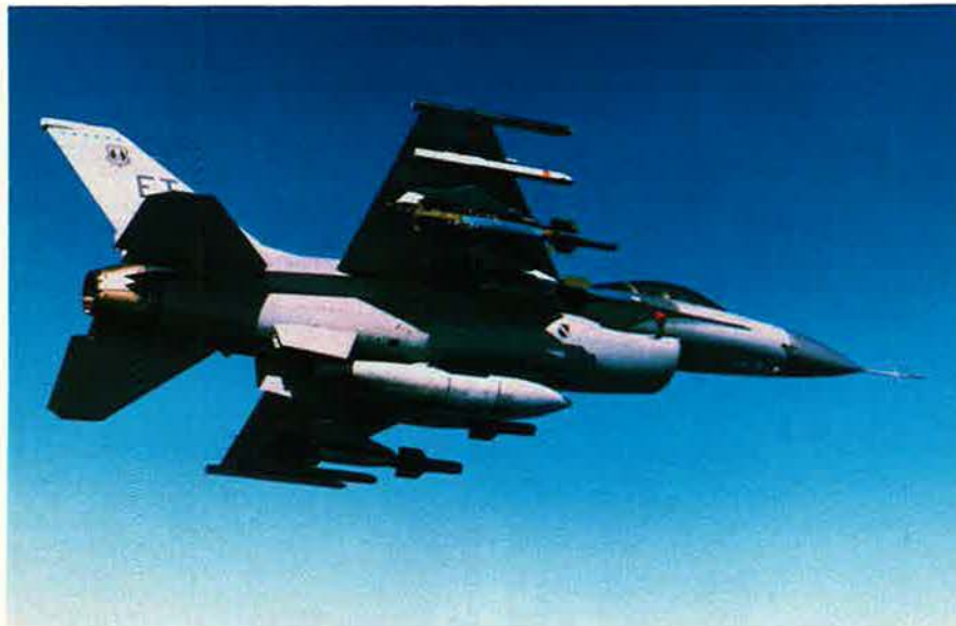
Texas Instruments successfully qualified use of the Paveway III laser-guided bomb GBU-22 on F-16 aircraft in tests conducted by USAF at Eglin AFB, Fla., from April to June. Funded by Texas Instruments, the test program included eleven flights, two of which were successful GBU releases.
