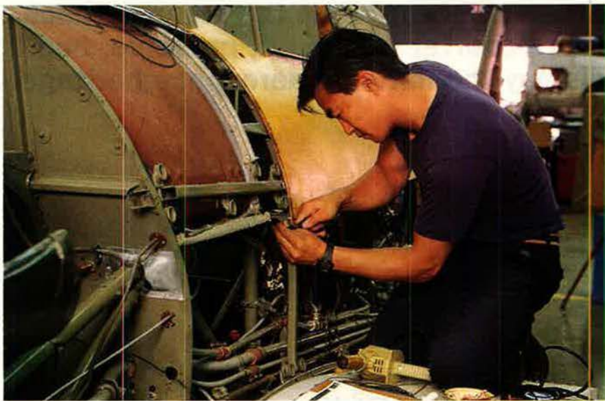
Admiral Engen says that he and Colonel Lopez agreed that the Garber restoration facility should "resume its eminent place in our hierarchy." Here, technician Will Lee works to restore a Hawker Hurricane.
