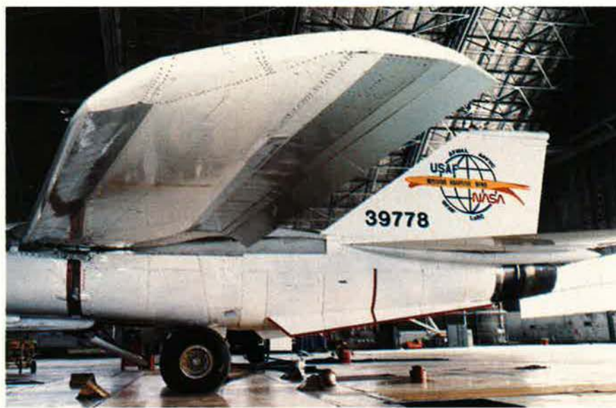
Ever since the Wrights discovered wing-warping, designers have manipulated the size and shape of wings for better performance, from the Berliner-Joyce XO-J1 with its "zap flaps" (top) to the Boeing-NASA-USAF F-111 with mission adaptive wing (above).
