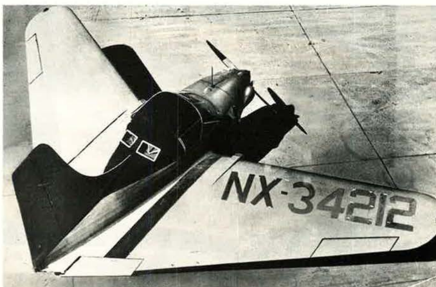
George Cornelius's 1930s-vintage "Mallard" (above) combined forward-swept wings with variable incidence. Grumman's highly successful X-29 technology demonstrator (top) had forward-swept wings whose trailing edges changed shape continuously to match flight conditions.
