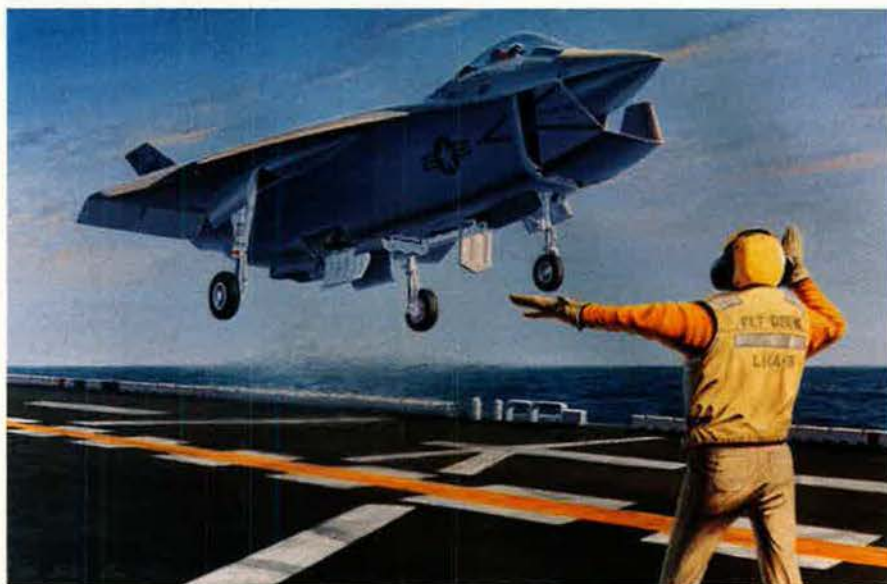
Boeing’s entry features an expandable inlet to gulp air for short takeoff and vertical landing operations. All JSF entries will be STOVL-capable, possibly paving the way toward smaller Navy carriers.
