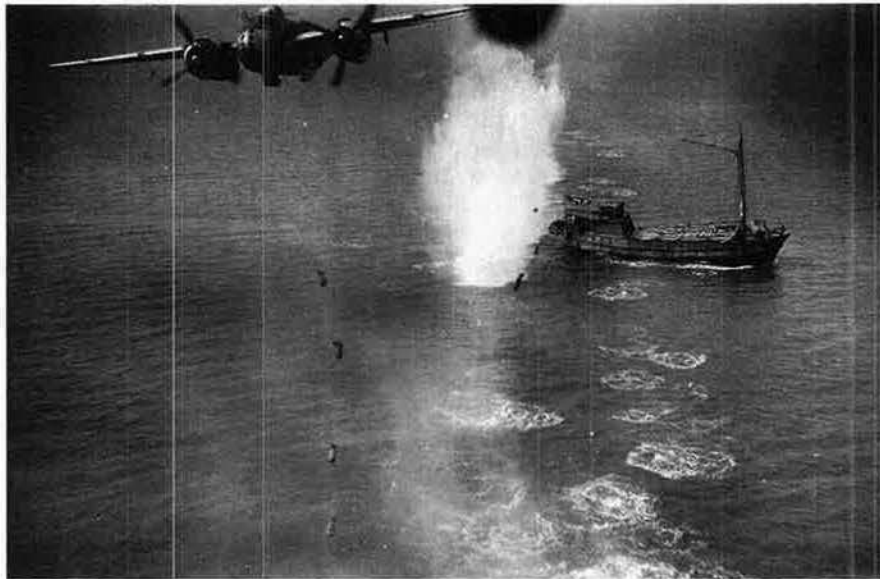
It was dangerous work, but modified B-25s were ideal for the task of cutting the enemy's supply lines. After skip bombing and strafing the deck, the bombers would hurdle the beset vessel, clearing the area before the bombs detonated.
