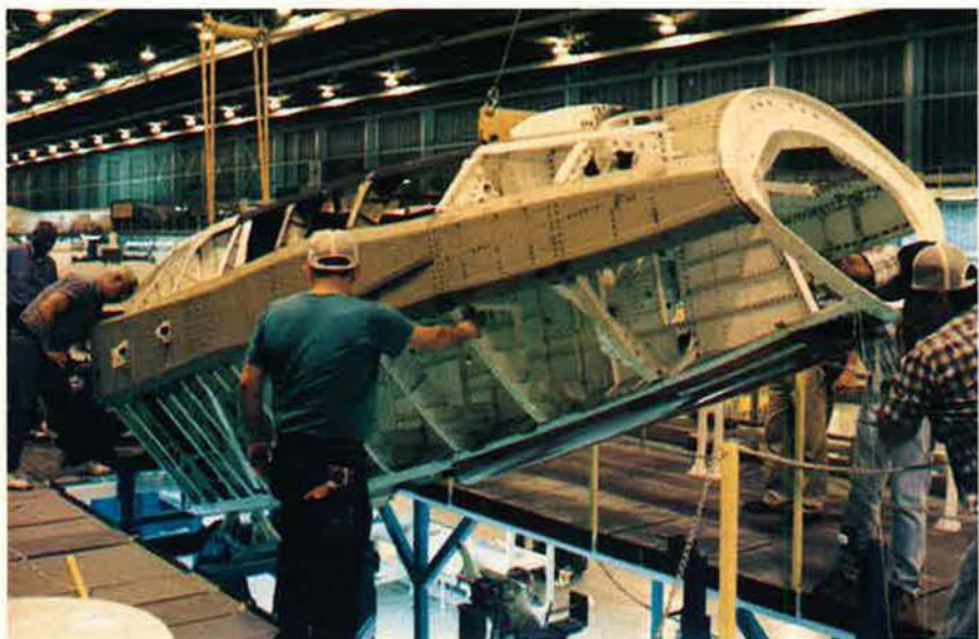
Lockheed Martin Aeronautical Systems, Marietta, Ga., recently completed another key step on the forward fuselage of USAF's first F-22. Major body mate—joining of the aft fuselage, built by Boeing in Seattle, Wash., to the mid-fuselage, built by Lockheed Martin in Fort Worth, Tex.—is scheduled for fall.
