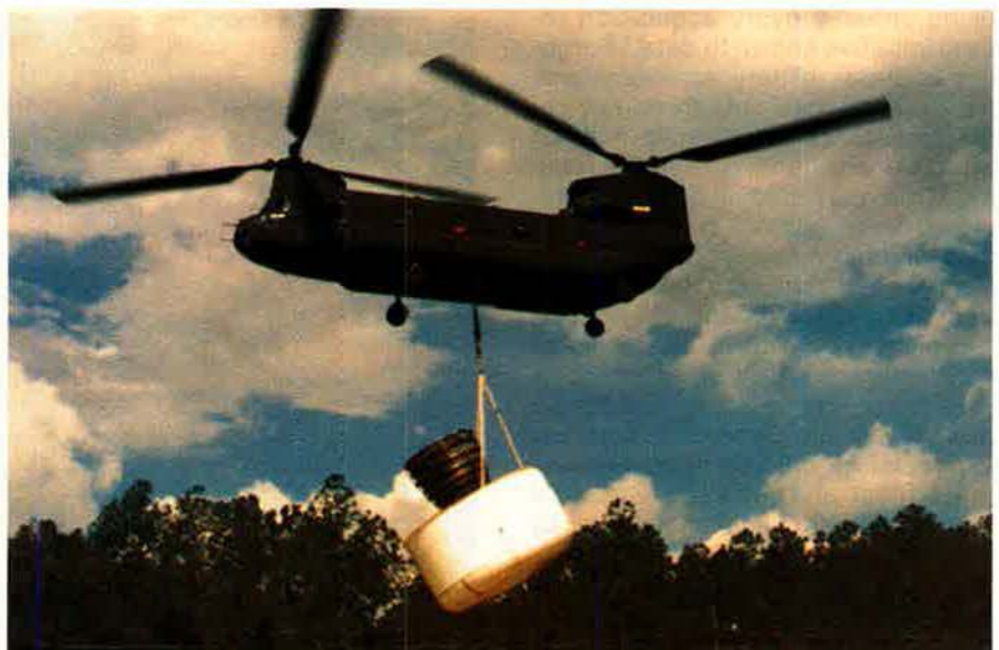
A Mississippi Army National Guard helicopter at NASA's Stennis Space Center helped conduct a lift test of the full-scale propulsion module for Boeing's "partially reusable" Evolved Expendable Launch Vehicle on June 7. The module would return to Earth for a parachute water landing after each launch.
