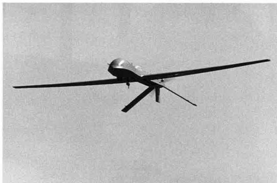
The Predator has seen extensive action over Bosnia, with more than 2,500 missions as of mid-May. At 450 pounds, its payload is more than quadruple that of the Pioneer. It also has a longer loiter time and higher maximum altitude.
