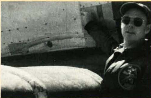
At Pyongyang AB (K-6), South Korea, in October 1951, Capt. Edward J. Monaghan points to the hole in his T-6 "Mosquito" made by a 12.7 mm bullet. The bullet hit a communications dynamotor, which exploded and damaged half the instruments in the cockpit and wounded Captain Monaghan, who went on to become an AFA national director. Lieutenant Colonel Monaghan, USAF (Ret.), presently resides in Anchorage, Alaska.
