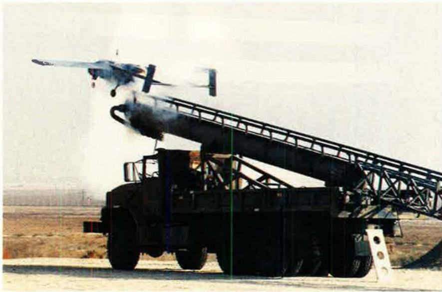
The Pioneer needs no airstrip, and it has seen extensive use already, including reconnaissance missions over the Persian Gulf, Haiti, Somalia, and Bosnia-Herzegovina. It has an action radius of 115 miles and can stay aloft for five hours.
