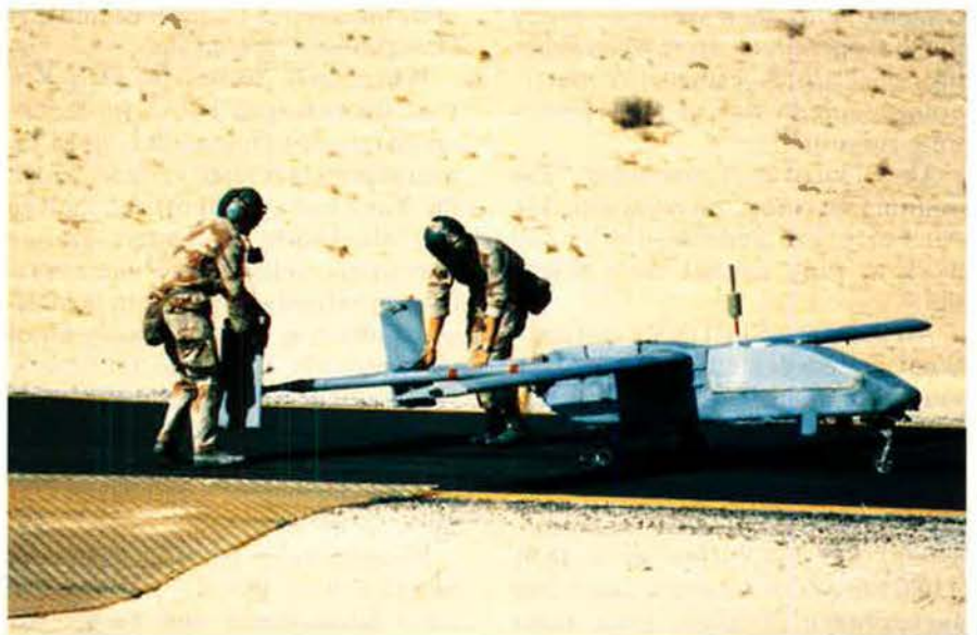
Formerly, remotely piloted vehicles like this one had to be controlled by "pilots" staring at a TV screen. The new generation of UAVs is much more autonomous, needing only the occasional progress check via mouse and keyboard.
