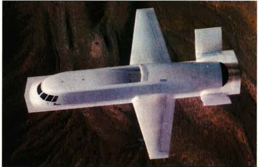
Tacit Blue, forerunner to today's stealth technology, shed its "supersecret" tag April 30, as the Air Force unveiled the $165 million program under contract to then-Northrop Corp. from 1978 to 1985. The single aircraft constructed (a second airframe shell served as backup) made 135 flights, beginning in February 1982. It had a 48.2-foot wingspan, was 55.8 feet long, and weighed 30,000 pounds. It is now on display at the US Air Force Museum in Dayton, Ohio.
