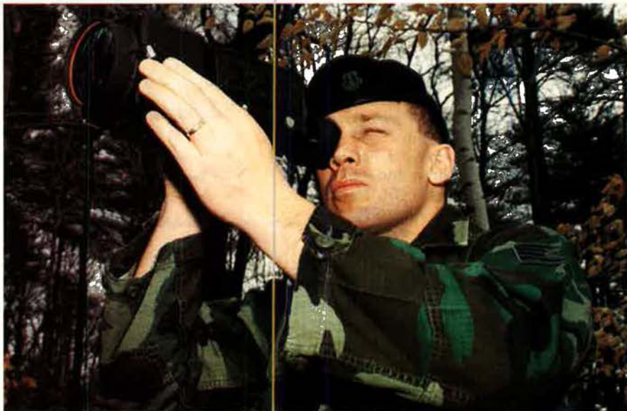
SSgt. Barry Lefavour, 66th Security Police Squadron, Hanscom AFB, Mass., demonstrates a handheld thermal imager that Hanscom's Electronic Systems Center officials say "sees" human silhouettes by detecting heat. USAF plans to purchase initially 230 units for Security Police forces.
