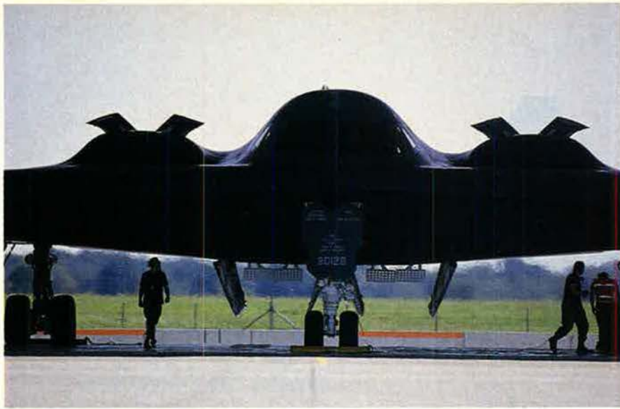
Engines keep turning as a Spirit changes pilots for another training sortie—a practice that eliminates the need for a lengthy preflight. The B-2's reliability has allowed crews to gain experience far faster than originally predicted.
