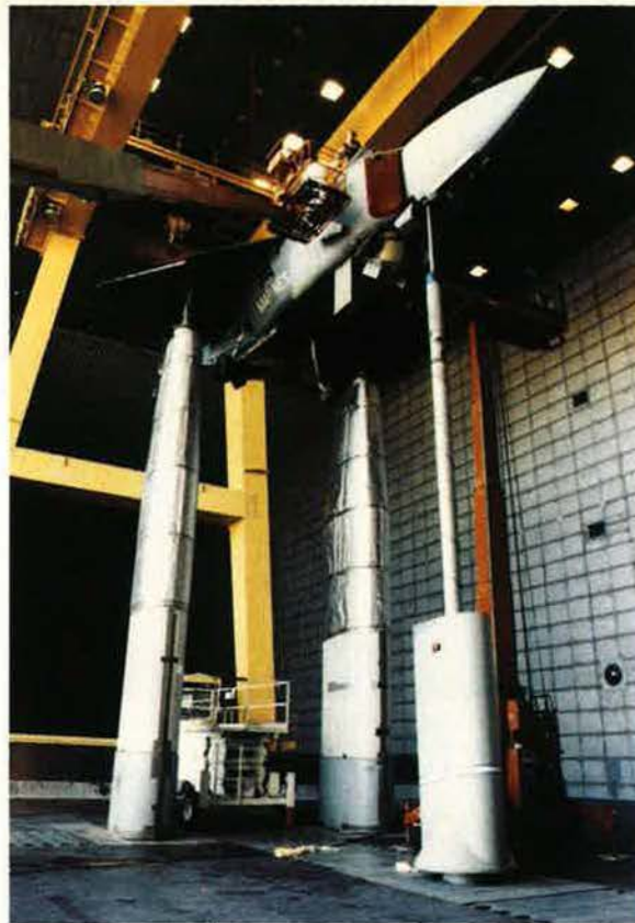
A large-scale powered model of Lockheed Martin's candidate for the future Joint Strike Fighter program undergoes wind tunnel testing at NASA's Ames Research Center. The JSF will be fielded by USAF, the US Navy and Marine Corps, and Britain's Royal Navy.
