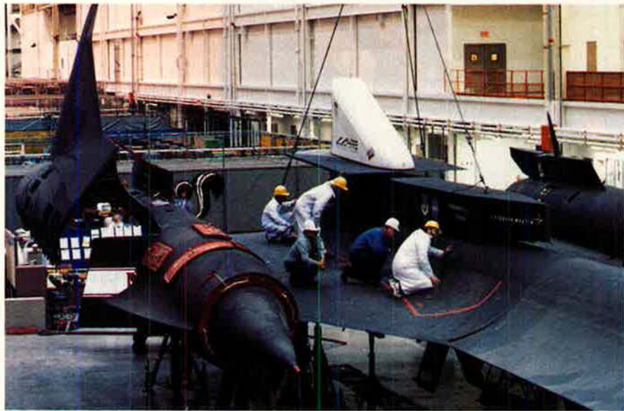
NASA, industry, and the Air Force are working together to develop a reusable launch vehicle to replace the space shuttle fleet. Above, a scale model of an RLV powerplant is fitted to an SR-71 "Blackbird" for testing at Lockheed Martin's "Skunk Works" in California.
