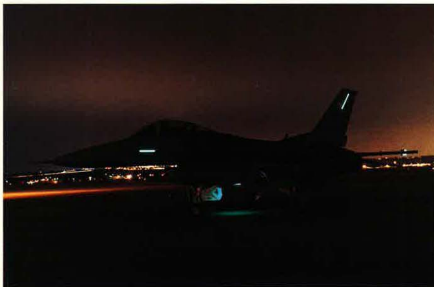
These luminescent strips will be visible only from above and beside Block 40 F-16s specially modified for night missions. The cockpit lighting was also extensively modified to make the F-16s compatible with the use of night vision goggles.
