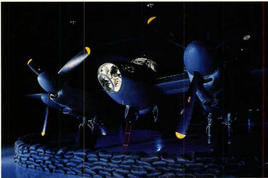
Constructed with "nonstrategic" building skills and crafted from molded plywood, the de Havilland Mosquito was very maneuverable and successful in many roles, from night fighting to photo-reconnaissance. The British-built light bomber is one of a dozen World War II-era airplanes on display at any given time in the Eagle Hangar, the museum's most popular wing. In describing this hall, EAA Executive Vice President Gregory J. Anderson says, "The Eagle Hangar collection presents the factual and inspirational context of ordinary individuals who did extraordinary things, from the home front to the front lines around the world."
