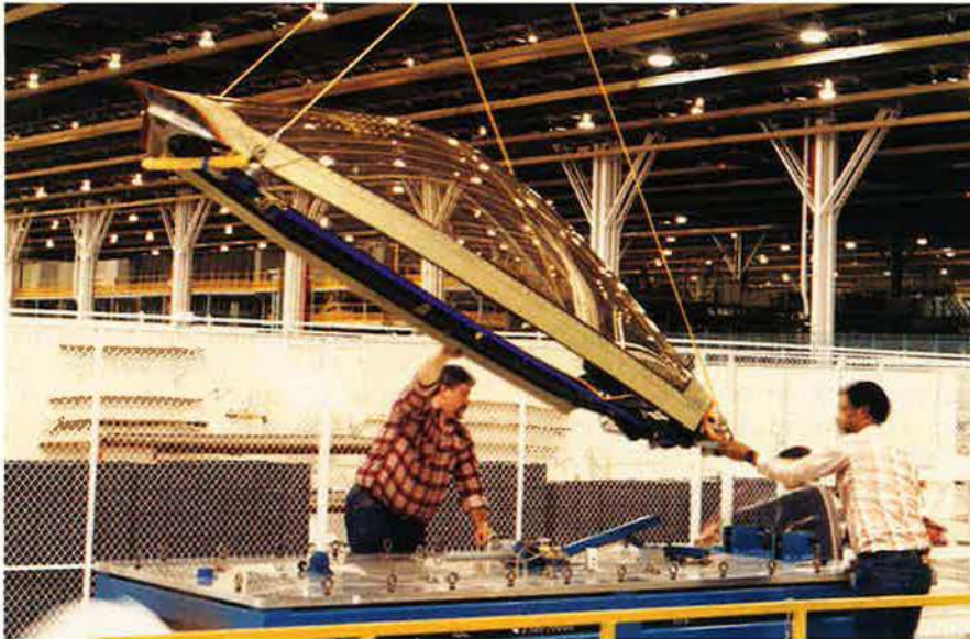
In January, Lockheed Martin technicians placed the first of seven F-22 test canopies into a test rig where it will be pressurized then checked for leaks. Program officials will use the canopies later this year to test the F-22's modified ACES II ejection seat.
