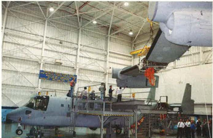
At Bell Helicopter Textron's Flight Research Center, Arlington, Tex., a crane moves the wing and nacelle structure of a V-22 Osprey into place on the aircraft's fuselage, signaling the start of final assembly. Bell Boeing officials say production of the tiltrotor aircraft is on schedule.
