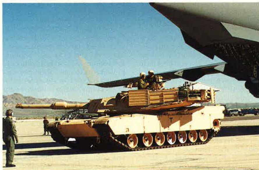
The C-17's ability to carry such outsize cargo as this M1A2 Abrams tank gave it the edge over the C-33, which also lacked roll-on/roll-off capability and could not operate on short or austere fields.
