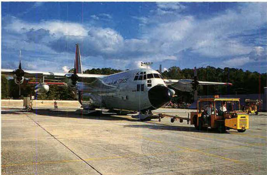
Lockheed Martin has produced seventy-four versions of the Hercules. Once an aircraft moves out of the plant, it is towed to the paint hangar. This factory-fresh LC-130H, with a special ski-and-wheel landing gear system, is headed for the 109th Airlift Group (ANG), Schenectady Airport, N. Y., which has an Arctic resupply mission.
