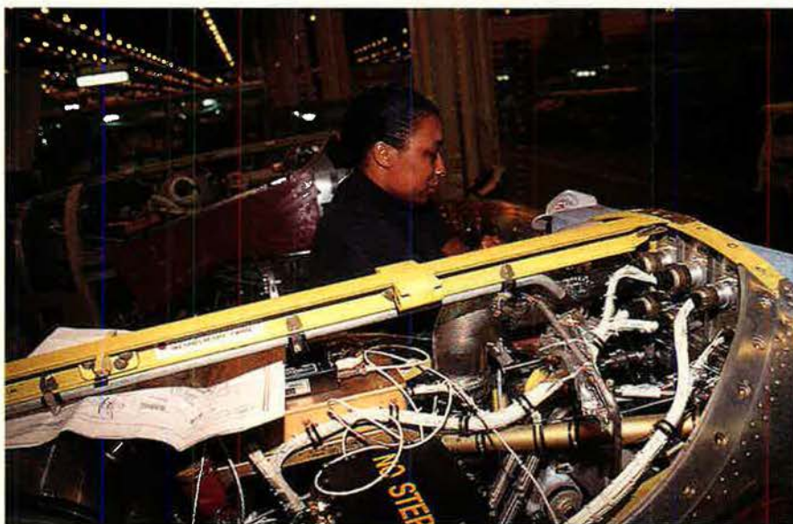
One of the next major steps is adding the engines. The C-130J has four new Allison AE 2100D3 engines that will be eighteen percent more fuel-efficient and will provide thirty-one percent more takeoff thrust. They also turn the transport's most visible new item—a Dowty Aerospace R391 all-composite six-blade propeller. The C-130J shares some technology with modern fighters: two mission computers, power-by-wire technology for the engines and propellers, and head-up displays for both pilots. At left, C. J. Stegall-Evans works on an Allison T56 engine before its installation on a C-130H.
