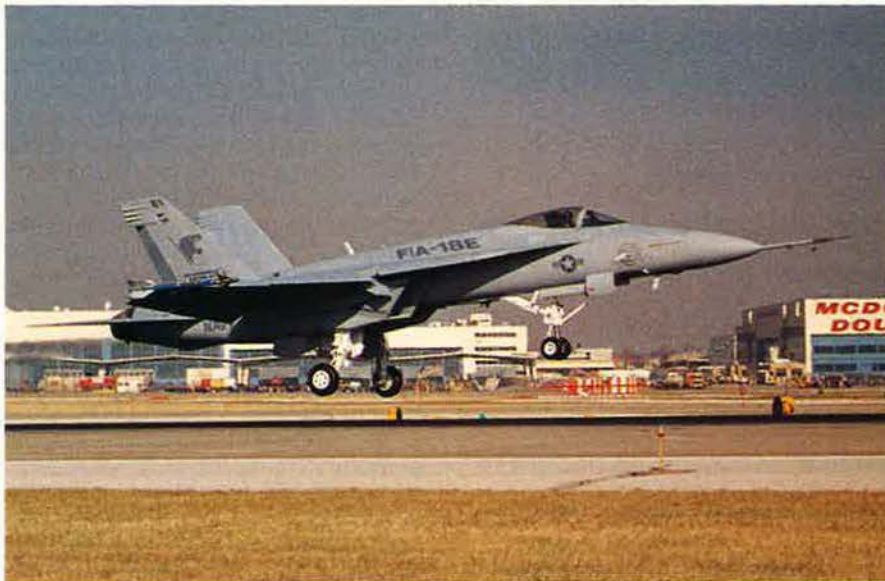
The Navy's new F/A-18E-F "Super Hornet" takes off on its first flight November 29. This latest version of the McDonnell Douglas aircraft is twenty-five percent larger, with longer range, greater endurance, increased weapons- and fuel-carrying capability, and improved survivability.
