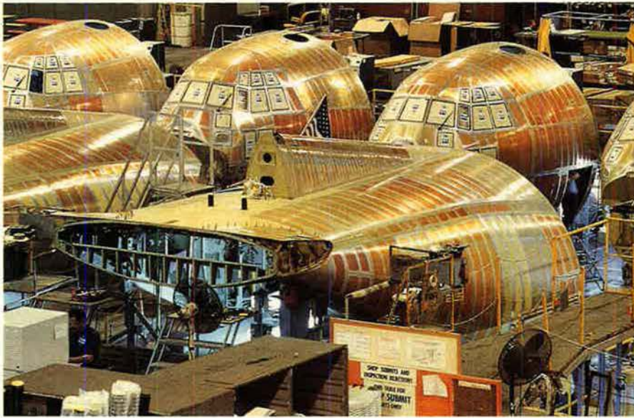
Feeder plants in Clarksburg, W. Va., and Meridian, Miss., produce some of the C-130J's components, such as the cargo bay floor, and subcontractors fabricate some parts, but most of the actual assembly takes place in the cavernous Plant Six. At left, a row of nose subassemblies faces a row of tail subassemblies. One of each will eventually be part of the same C-130, separated by about 100 feet of aircraft.
