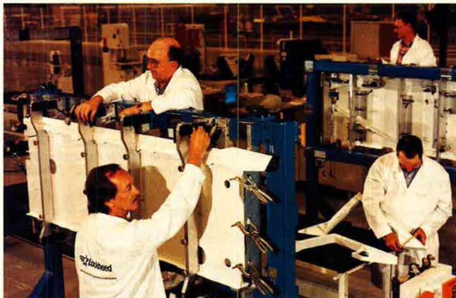
Assembly of USAF's first F-22 fighter started on schedule November 2 as Lockheed Martin workers in Marietta, Ga., began connecting elements of the nose landing gear wheel well, part of the forward fuselage. In all, the well consists of 168 parts.
