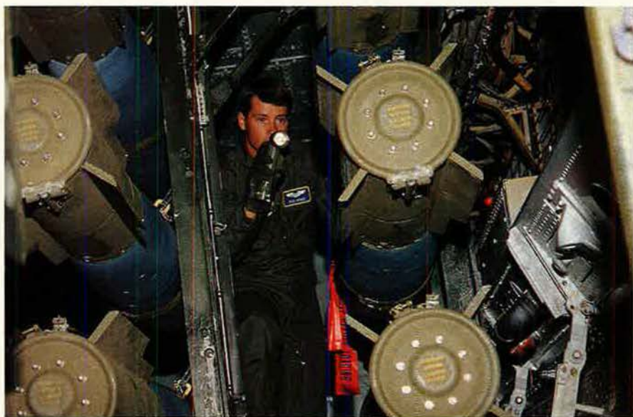
Fully loaded, the B-52 can carry more than 70,000 pounds of weapons, including the 500-pound Mk. 82 high-drag bombs that radar-navigator Capt. Tray Hodge of the 20th Bomb Squadron checks here during his walkaround. With packing, preparation, and walkarounds by various crew members, it will be another thirty minutes before engine start for this B-52.
