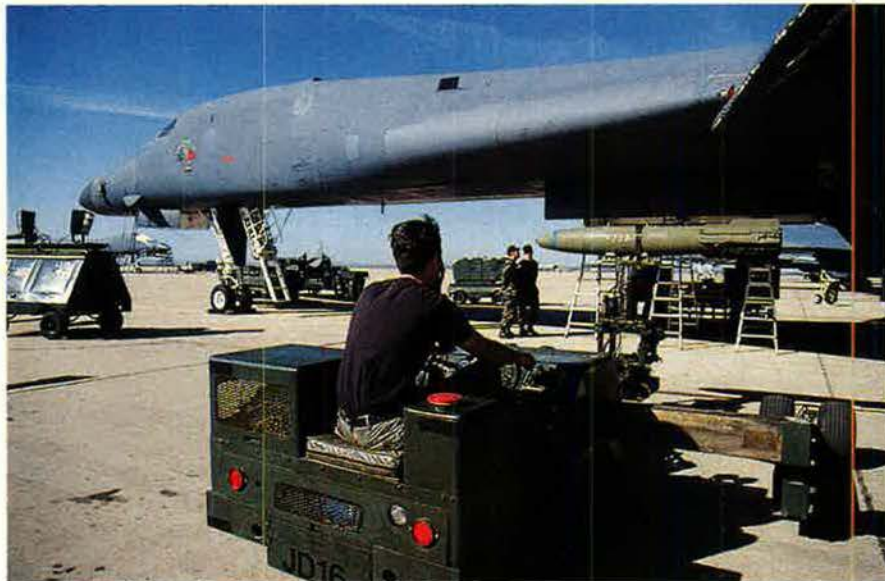
The B-1's capability will grow significantly with such new precision weapons as JDAM, but speed and load make it a formidable conventional platform today. It can deliver eighty-four 500-pounders anywhere within twenty hours.
