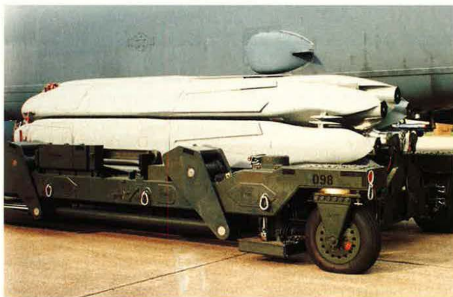
Among the developments that extended the B-52's functional life were the cruise missile, seen here on the bomb-bay Common Strategic Rotary Launcher, and the GPS antenna. B-52s released some of the first weapons of the Gulf War.
