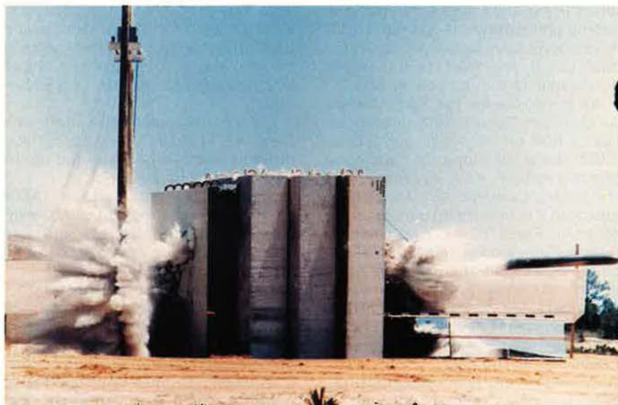
USAF completed operational tests in March on Texas Instruments' improved "bunker buster," used in Operation Desert Storm. Above, the BLU-113A/B "business end" of the GBU-28A/B laser-guided bomb penetrates fifteen feet of steel-reinforced concrete during a qualification sled test at Eglin AFB, Fla.
