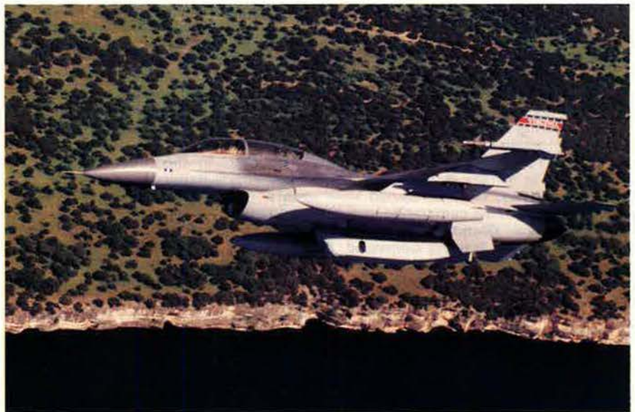
An Air National Guard F-16C from the 192d Fighter Group, Richmond, Va., evaluated an off-the-shelf Lockheed Martin-designed electro-optical pod configuration on April 26 as part of the first step in transferring the manned tactical reconnaissance mission from the RF-4C to the F-16.
