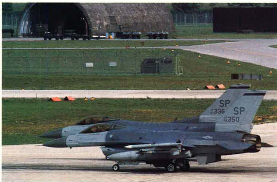
More with less: USAFE F-16s have been enhanced to pack more missions into fewer airframes. New capabilities include Advanced Medium-Range Air-to-Air Missiles and Low-Altitude Navigation and Targeting Infrared for Night capability.
