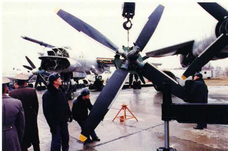
In April, Defense Secretary William J. Perry toured the Engels Heavy Bomber Base, 520 miles southeast of Moscow, Russia, where sixty-four Tu-95 strategic bombers have been destroyed under Strategic Arms Reduction Treaty provisions. Here, a propeller assembly is removed to "demilitarize" a bomber.
