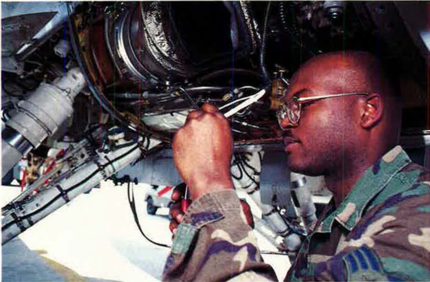
With the wing called on to respond to an increasing number of contingencies, maintenance and repair are more important than ever to unit readiness. At left, SrA. Cedric Weatherspoon, an electro-environmental systems journeyman with the 69th FS, splices wires on a door switch harness.
