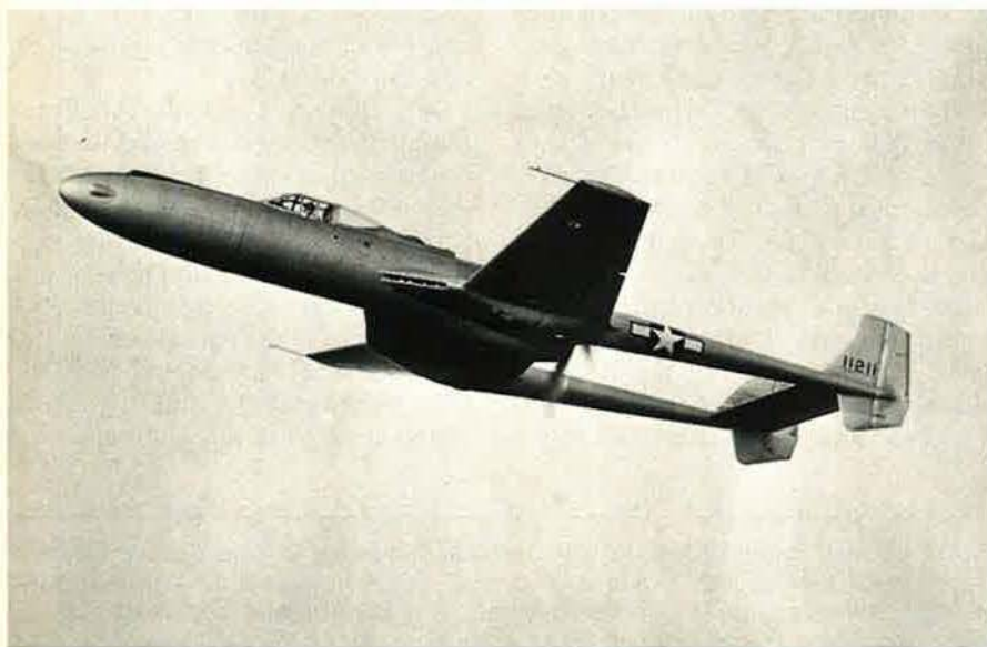
An early type of American ejection seat appeared in the Vought XP-54 Swoose Goose. The pilot entered the aircraft from the bottom fuselage, on a seat that raised him into the cockpit. In an emergency, it reversed to catapult him away.
