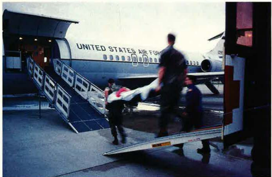
The C-9 Nightingale medical evacuation aircraft, originally designed to transport as many as forty fairly stable patients along with up to five medical personnel, has worked well for USAF since 1968 with few major changes.
