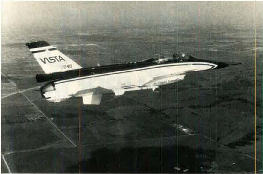
The VISTA/NF-16D employs a production F-16D airframe, with features from different F-16 variants, plus a complex, custom-designed variable stability system. Materiel Command's Wright Laboratory will use the aircraft to simulate other aircraft, perform aeronautical research, and train new military test pilots.
