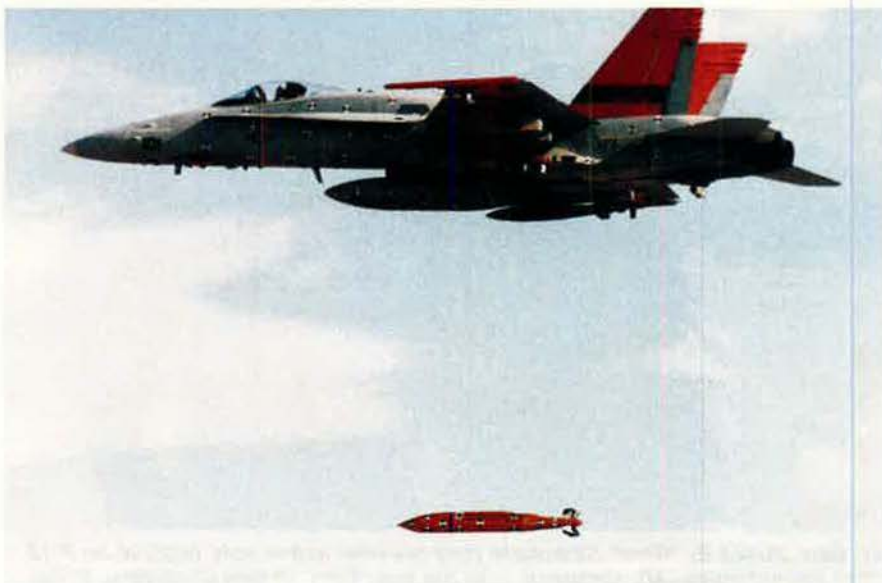
Texas Instruments announced successful completion of the first Joint Standoff Weapon (JSOW) guided free-flight test, using a US Navy F/A-18C on December 13. JSOW is a low-cost, standoff weapon developed with Naval Air Systems Command to provide an affordable, multipurpose standoff attack capability.
