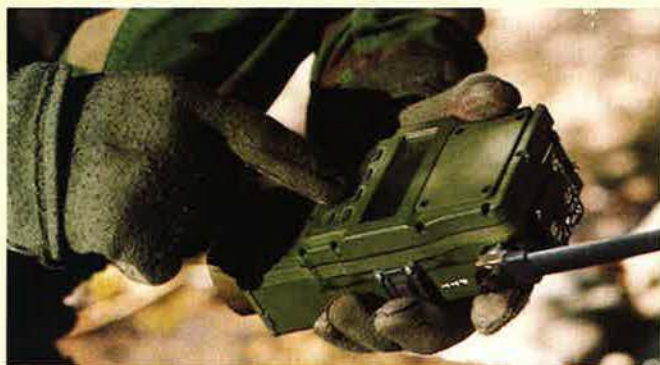
GPS-112 Search and Rescue Handheld Transceiver
