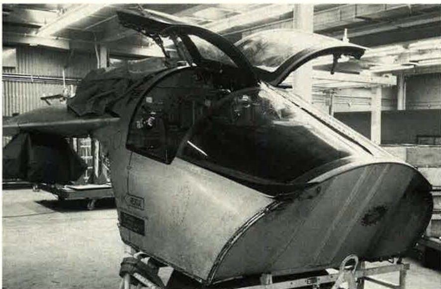
USAAF's first live, in-flight ejection took place in 1946 at 228 knots and 7,800 feet. In 1968, two General Dynamics crewmen in this McDonnell Douglas module landed unhurt after being ejected at 29,000 feet over Texas at Mach .87.
