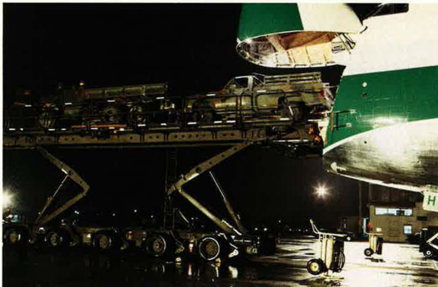
Boeing proposes to build a 747-400 with hardened decks, a side-loading door, and a flip-up nose. Cargo could be lifted into the aircraft on scissors-type platforms, which are used in civilian aviation around the world.
