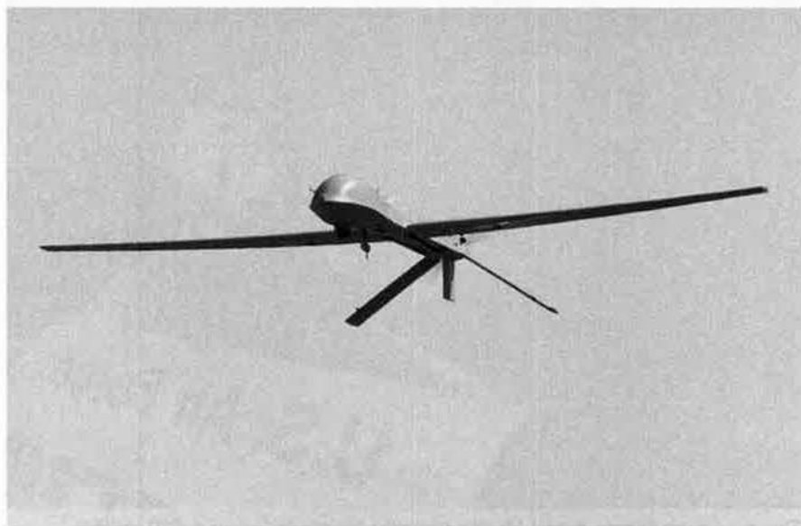
Promising expanded range, endurance, and payload capacity, General Atomics Aeronautical Systems, Inc.'s Predator Tier II (above) is in flight testing along with another high-performance unmanned surveillance aircraft, the Gnat-750.
