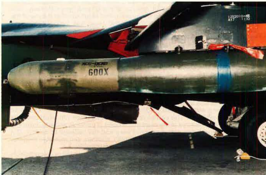
Rockwell International Corp.'s GPS/INS guidance unit was found to reduce pilot work load and improve weapon effectiveness in simulated missile flight profiles. Fifty-nine flight tests have been completed aboard an AGM-130 missile mounted on an F-111 at Eglin AFB, Fla.
