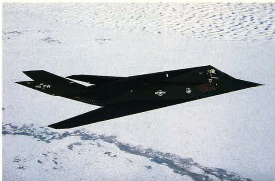
Thanks to advances in composite material development, F-117 trailing edge parts are now fabricated out of a new resin, which is not only harder to damage but can withstand higher temperatures.
