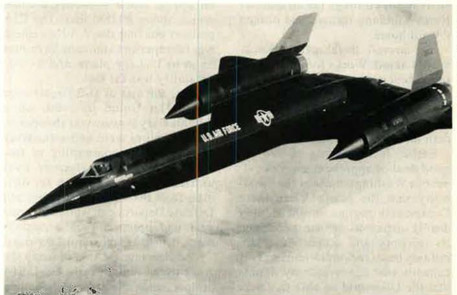
The A-12 reached its top cruising height above 90,000 feet in a hurry with its Mach 3-plus speed. Once there, it had a range of more than 3,000 nautical miles. At that altitude and speed, it was safe from most threats.
