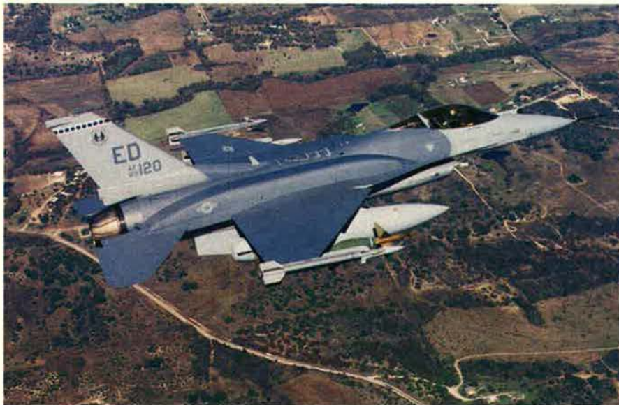
Lockheed's "enhanced strategic" F-16 fighter, fitted with mock conformal fuel tanks (mounted above the wings), two 2,000-pound laser-guided bombs, two AMRAAMs, and two AIM-9 missiles, demonstrates its handling in test flight.
