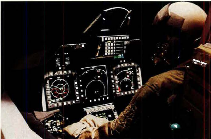
Not all of Air Force Materiel Command's experimental technologies pay off. Testing high-tech touch-sensitive display screens in the F-22 cockpit, for example, revealed that pilots prefer old-fashioned buttons.
