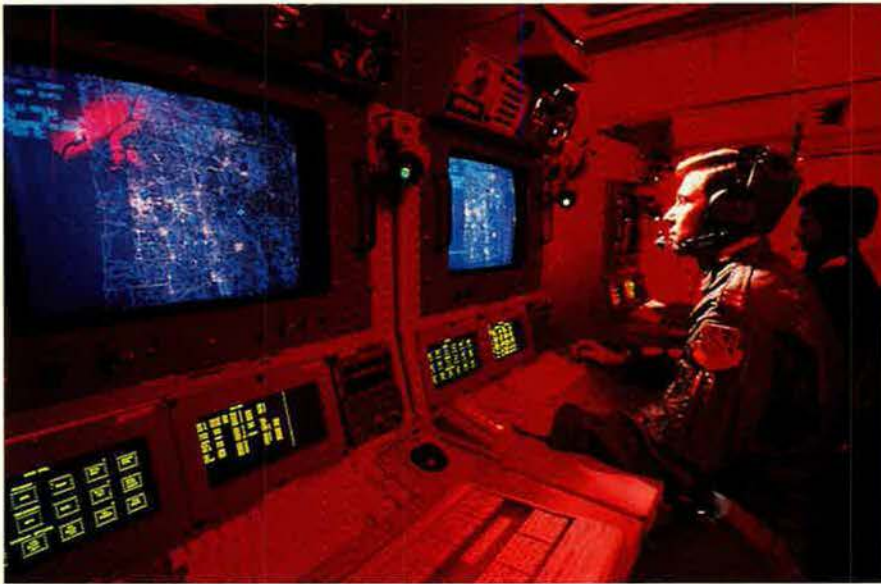
The E-8 Joint Surveillance and Target Attack Radar System's sophisticated technology can detect enemy command centers and distinguish a mobile missile launcher from a decoy. Detailed, color-coded images appear on-screen . . .
