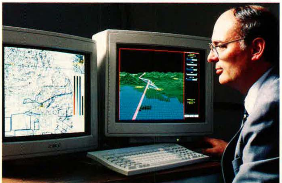
The AFMSS will permit side, forward, and rearward views, as well as split-screen displays. The right screen here shows a three-dimensional view of a flight path while the left adds threat information and navigation charts.
