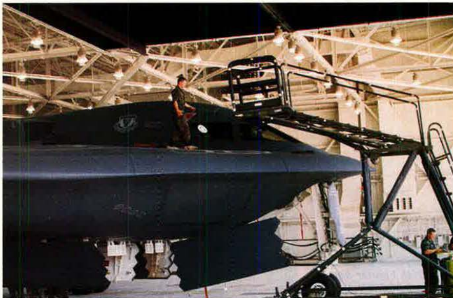
The first operational B-2, Spirit of Missouri, undergoes its first phase inspection, a maintenance check performed after every 200 flying hours. After the check, members of the 509th Maintenance Squadron may spend as much time restoring the plane's stealth characteristics as they did on maintenance.
