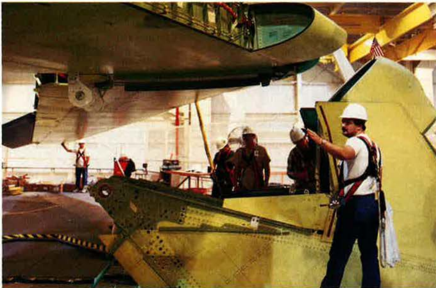
McDonnell Douglas has focused on rectifying C-17 management and production problems. Above, a horizontal stabilizer is attached to a C-17's vertical stabilizer at the company's Long Beach, Calif., plant.
