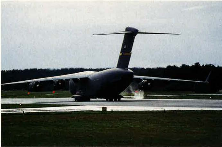
A C-17 whips up air currents as it demonstrates its thrust-reverse and short-field takeoff abilities. By Air Force calculations, the Globemaster III can use many more runways around the world than the C-5 can.
