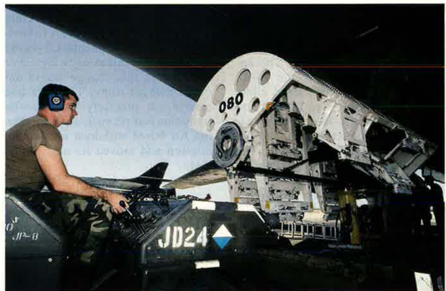
A technician moves a conventional modular bomb rack into position in the B-1B's internal weapons bay. ANG ground crews have been working on the "Bone" alongside their active-duty counterparts every day since March.
