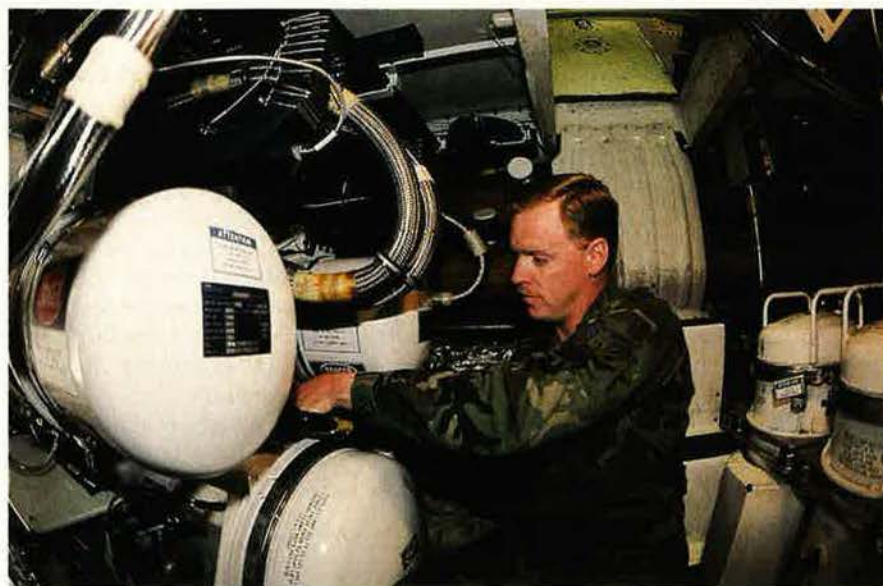
SrA. Cory Petty examines a radar transmitter component in an E-3. Upgrades will enable the E-3's radar to detect aircraft with one-tenth the signature visible to today's radars, allowing the aircraft to spot tiny Cessnas and cruise missiles.
