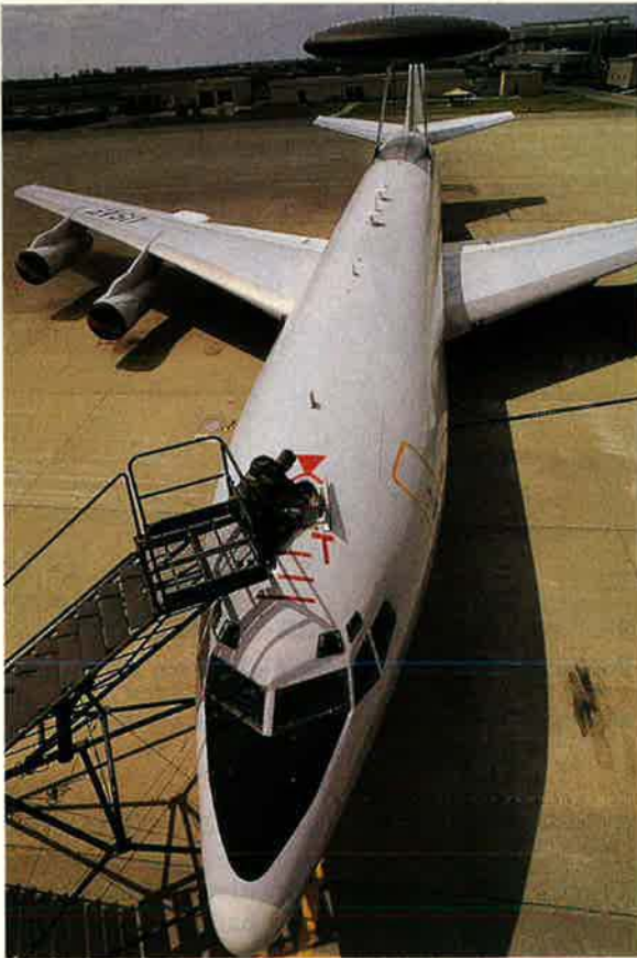
Both the E-3 (left) and the E-8 Joint STARS are based on the Boeing 707 airframe, which is no longer in production. Some E-3 customers have moved to the Boeing 767 as a platform. E-8 procurement officials are scouring the world for used 707s capable of the Joint STARS mission.
