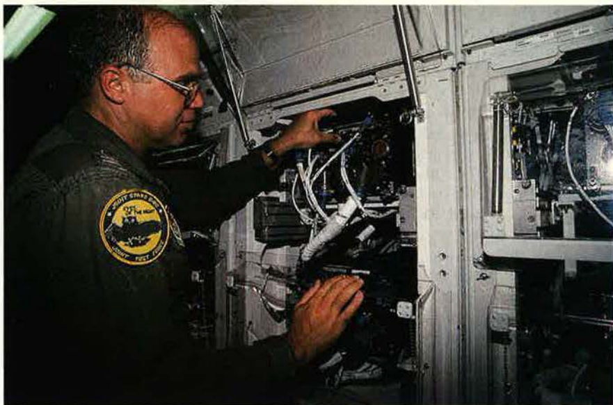
Capt. Carl Mallette checks an E-8's electronics at Northrop Grumman's Melbourne, Fla., facility. Joint STARS radars can cover almost 400,000 square miles of ground territory in a single eight-hour sortie.
