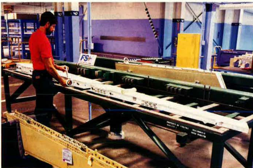
Lockheed assembly mechanic Larry Rutledge works on the first leading-edge wing flap completed for the FS-X aircraft program. Lockheed is producing sixteen of these flaps for Mitsubishi Heavy Industries of Japan.
