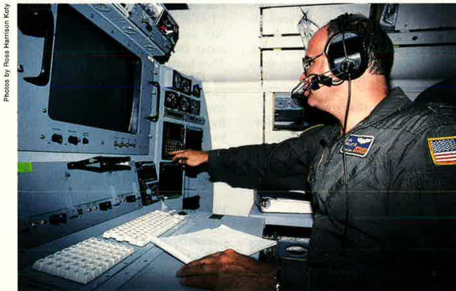
Captain Mallette, a member of the Joint STARS combined test team, checks data at one of the E-8's ten operations consoles. Joints STARS will have direct links to ground forces and the US command-and-control structure.
