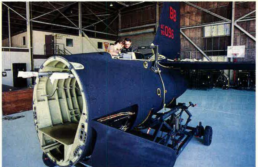
SrA. Dawne Chance and TSgt. Bob Phillips, avionics technicians, go over the tail section of a U-2. This up-close look at the U-2's internal structure shows its extended air brakes and ultralight construction.
