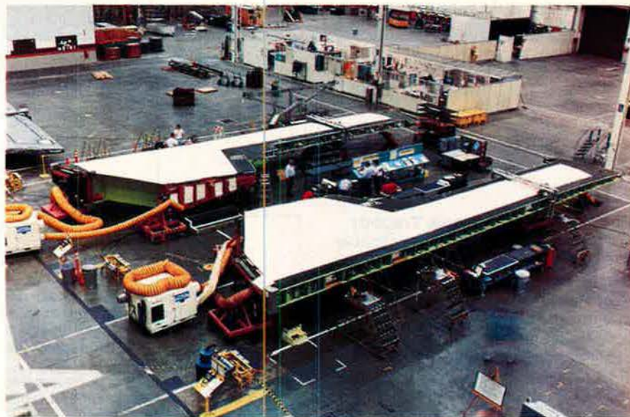
Boeing Defense & Space Group completed assembly of the outboard wing sections for the Air Force's twenty-first B-2 bomber (including the prototype) in May. The sixty-five-foot sections are believed to be the largest structural aircraft parts ever made from composite materials.
