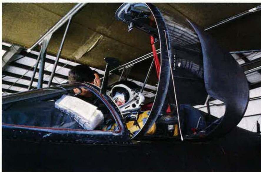
Specialized life-support technicians keep a close watch on a U-2 pilot all the way into his airplane. Here, a technician hooks up Colonel Lloyd to his support systems just before he begins a high-flight training mission.
