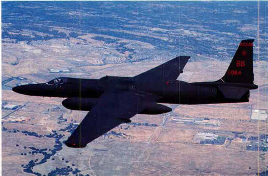
In flight, the sleek, black U-2 is a study in grace, whether soaring over San Francisco's Golden Gate Bridge (previous pages) or the countryside of northern California (above). Two underwing "superpods" carry some of its sensors.
