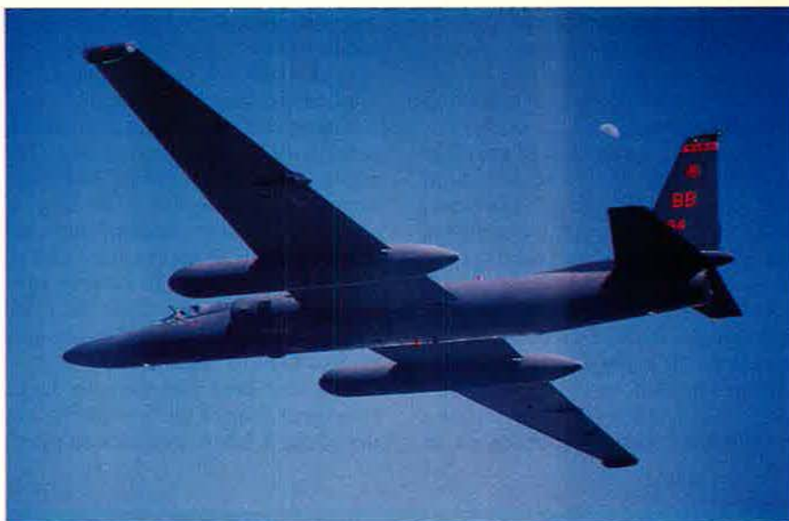
The U-2 performs not only photo intelligence but also radar intelligence, electro-optical signal analysis, and electronic intelligence. The U-2R can perform such nontraditional tasks as air sampling for radiation.
