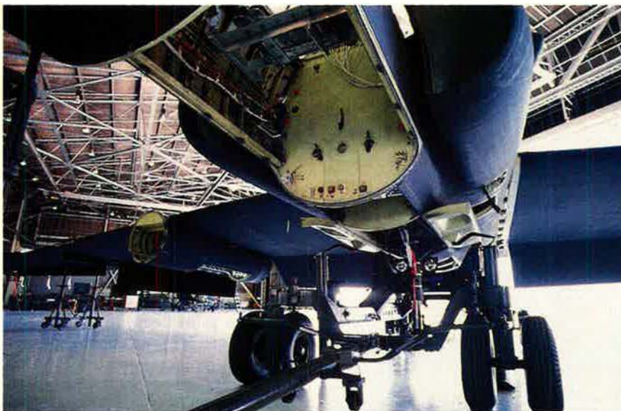
Another view of the U-2 provides an excellent look at the aircraft's Q-bay, location of cameras and sensors. Additional surveillance and reconnaissance equipment can be installed using superpods hung beneath the wings.
