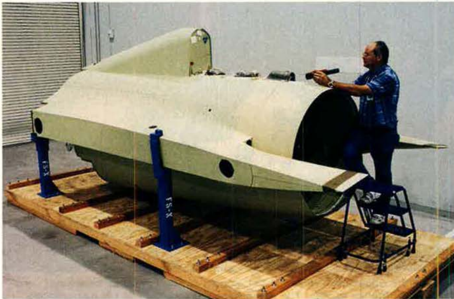
A Lockheed quality inspector examines the first aft fuselage section for an FS-X flight test aircraft. Mitsubishi Heavy Industries, the Japanese prime contractor for the F-16 derivative, will assemble the aft section with other airframe components to complete the first prototype. First flight is scheduled for mid-1995.
