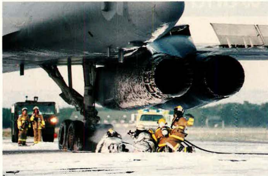
A B-1B bomber crew from the 9th Bomb Squadron, 7th Wing, Dyess AFB, Tex., was forced to land at Rhein-Main AB, Germany, with the bomber's wings swept back after they would not go to cruising position. The aircraft touched down at 242 knots and blew four landing gear tires. No injuries were reported.
