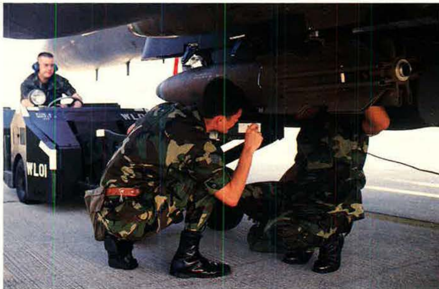
A Mk. 82 500-lb. gravity bomb is loaded on an F-15E at Eglin AFB. As the Gulf War showed, it takes too many unguided dumb bombs to destroy too few targets. What USAF needs instead are autonomously guided, all-weather weapons.
