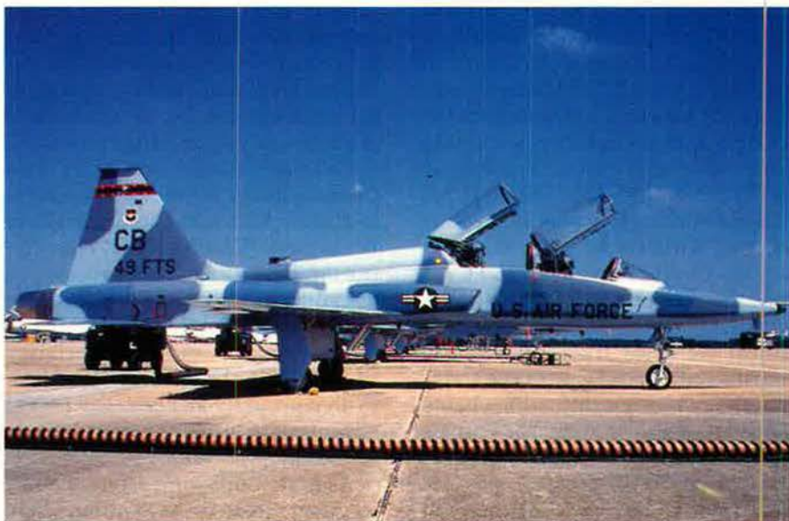
AETC's Introduction to Fighter Fundamentals is a short, difficult course using AT-38 Talons equipped with gunsights and practice bomb dispensers. This AT-38B is at Columbus AFB, Miss., where AETC's first IFF class graduated in 1993.
