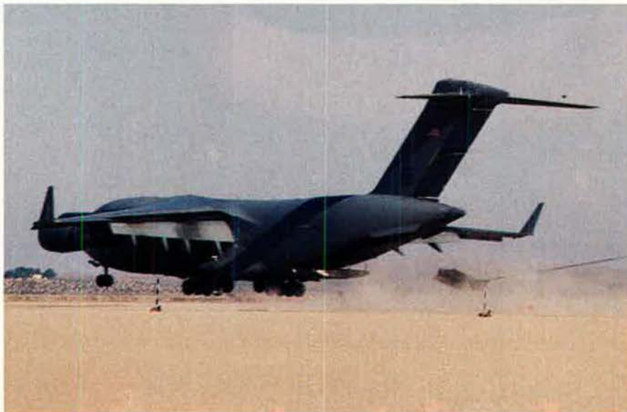
A McDonnell Douglas—USAF C-17 successfully made its first aerial delivery using the low-altitude parachute extraction system in May. In this test of combat delivery of heavy loads, a 6,700-pound test platform was extracted from the aircraft as it flew at 150 mph, two feet above the dry lake bed at Edwards AFB, Calif.
