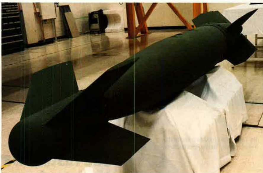
A Mk. 83 1,000-lb. bomb becomes a Joint Direct Attack Munition (shown in this mockup) when a JDAM guidance kit turns it into a precision guided munition. Like the new PGMs, new munition dispensers, such as the one opposite, on an F-16C at Eglin AFB, Fla., are expected to work wonders for airpower.
