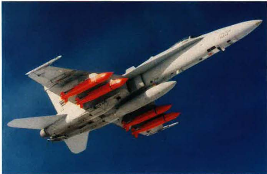
The Navy F/A-18 fighter bristles with Joint Standoff Weapons, developed by Texas Instruments for the Navy and USAF. JSOW, which sprouts wings and flies forty miles, can carry munitions, mines, or warheads for various missions.
