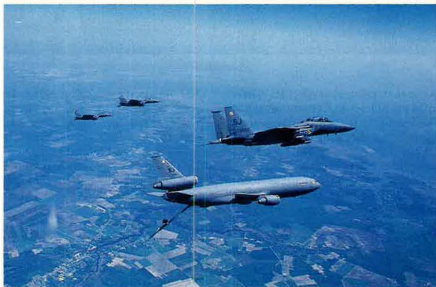
Four aircraft approach the tanker track of a KC-10 from the 344th ARS of the 4th Wing. Radar and forward-looking infrared are used to identify the tanker from afar. An F-15E (top) uses its airbrake to bleed off speed.
