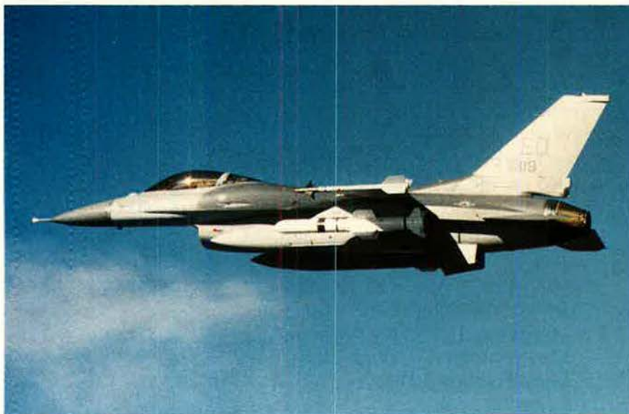
Flight testing of the AGM-84 Harpoon antiship missile on the F-16 began in March at Edwards AFB, Calif. The testing will verify avionics systems integration of missile and aircraft. Lockheed Corp. produces the F-16, and McDonnell Douglas produces the Harpoon, the standard US antiship missile.
