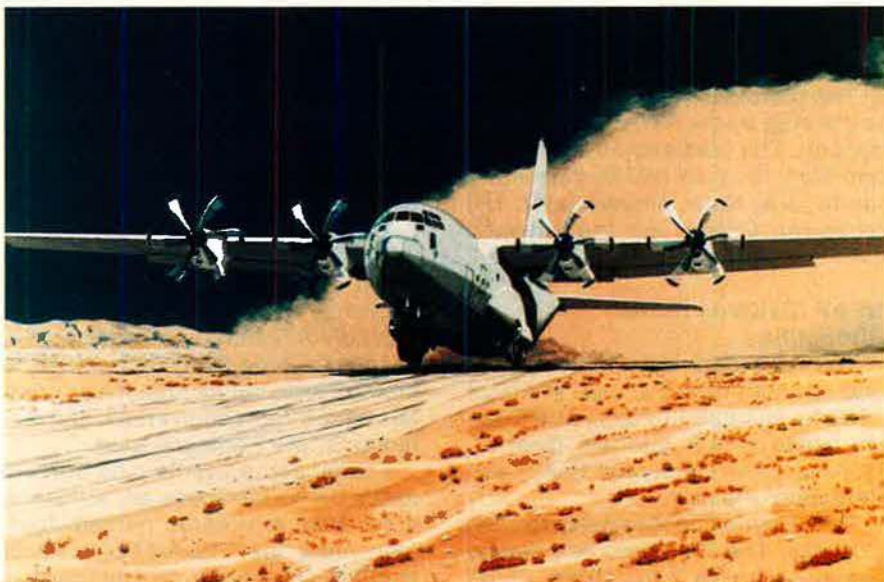
In March, Lockheed Aeronautical Systems Co. fabricated the first parts for the new C-130J, scheduled for rollout in mid-1995. One obvious change to the C-130J is the six-blade propellers on each of its four engines. The J will have the versatility and airlift capability of its predecessors but with improved performance.
