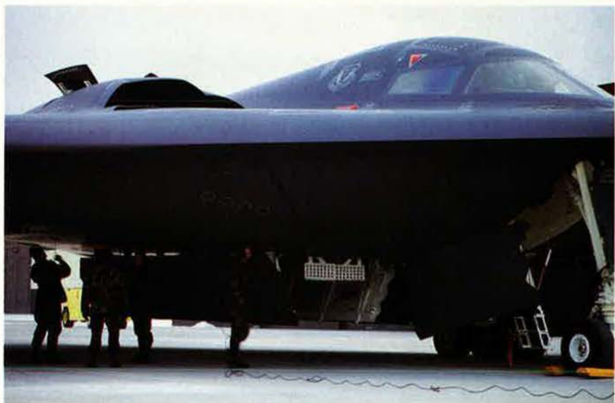
Aircraft maintainers assisted B-2 designers. Easy access to compartments was a happy result. B-2 compartment doors fit so snugly that they are constantly sharpened like scissors. Ground crews put safety guards over the door edges.
