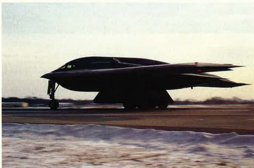
This view of the B-2 accelerating down the runway illustrates some of its design complexity. Its trailing-edge control surfaces make up about fifteen percent of total wing surface. Note the huge nose gear and main landing gear door.
