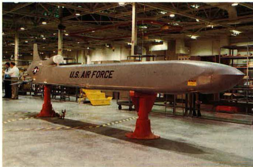
Virtually indistinguishable from its nuclear-armed counterpart, the AGM-86C instead carried a 1,000-pound conventional blast fragmentation warhead, which struck with the effectiveness of a 2,000-pound bomb.
