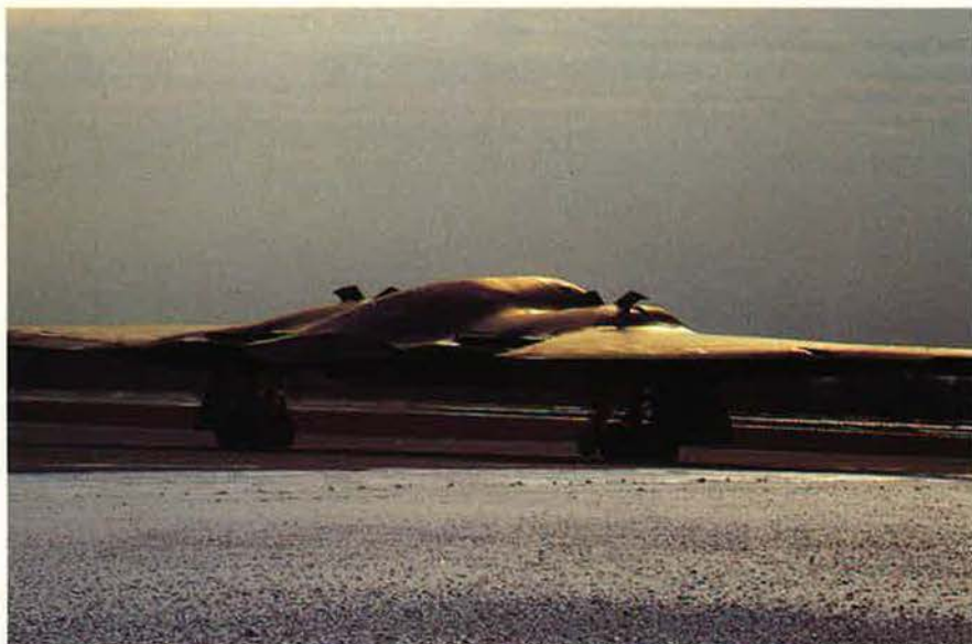
Blended surfaces characterize the huge flying wing. Nearly as great in wingspan as the B-52, the B-2 is slightly longer than the F-15. With its lack of tail and widely spaced landing gear, the B-2 represents a new era in aircraft design.
