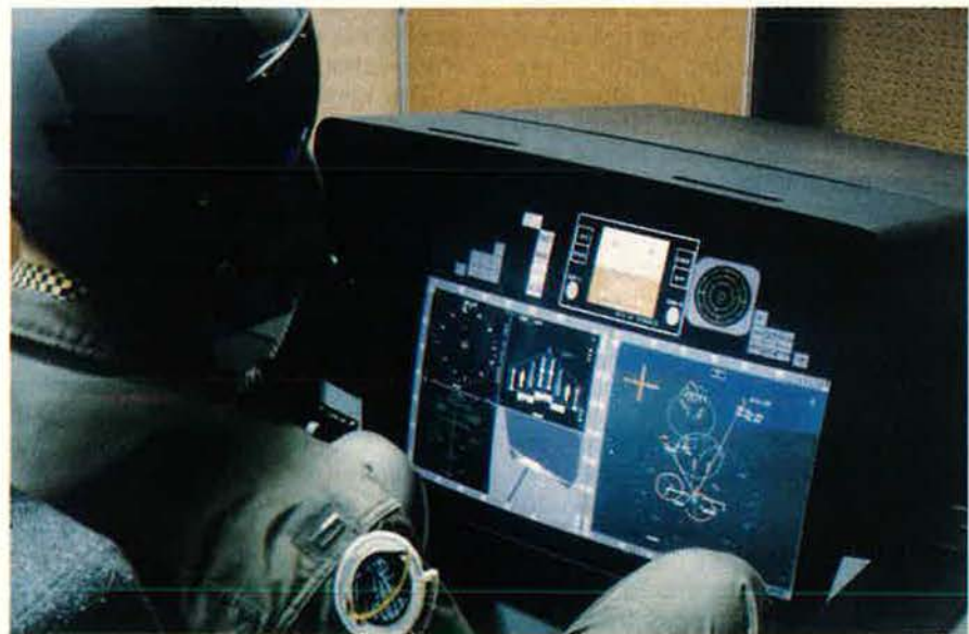
The Integrated Mission Precision Attack Cockpit Technology program at Wright Laboratory, Wright-Patterson AFB, Ohio, tests air-to-ground technologies that will enable one pilot to perform missions that take two in some fighters.
