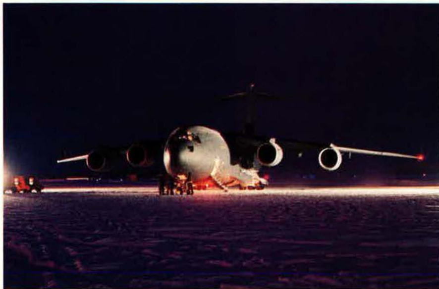
The C-17 "P-3" was deployed to Eielson AFB, Alaska, for cold-weather testing in January and flew over the North Pole in February. The polar mission set a record for the longest C-17 flight, 8.7 hours.
