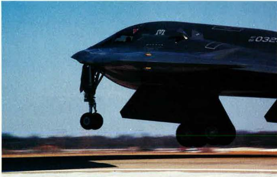
The B-2 takes off, showing the variation in camber of the leading edges. After extensive and realistic simulator and classroom work, pilots are expected to "know everything about the aircraft," says B-2 IP Lt. Col. Tony Imondi.
