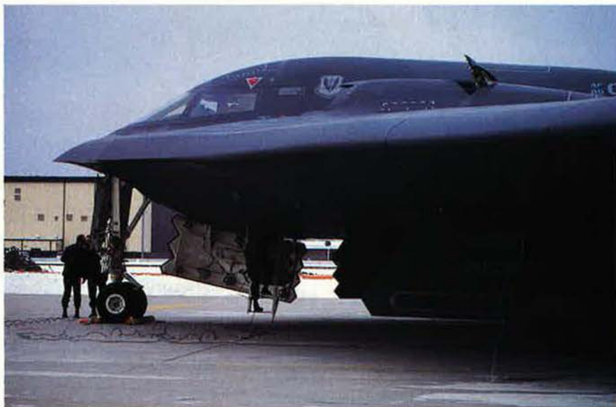
Note the auxiliary intake door atop the B-2's engine nacelle. Two doors in each nacelle provide optimum mass airflow to the engines at idle. Below, a crew chief communicates with pilots during preflight.
