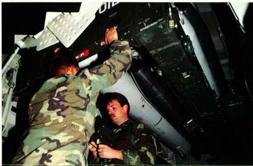
Crew members work in the B-2 Weapons Load Trainer. Such training systems help prepare crews for work on the actual aircraft. The B-2 uses rotary launchers for both conventional and nuclear weapons delivery.
