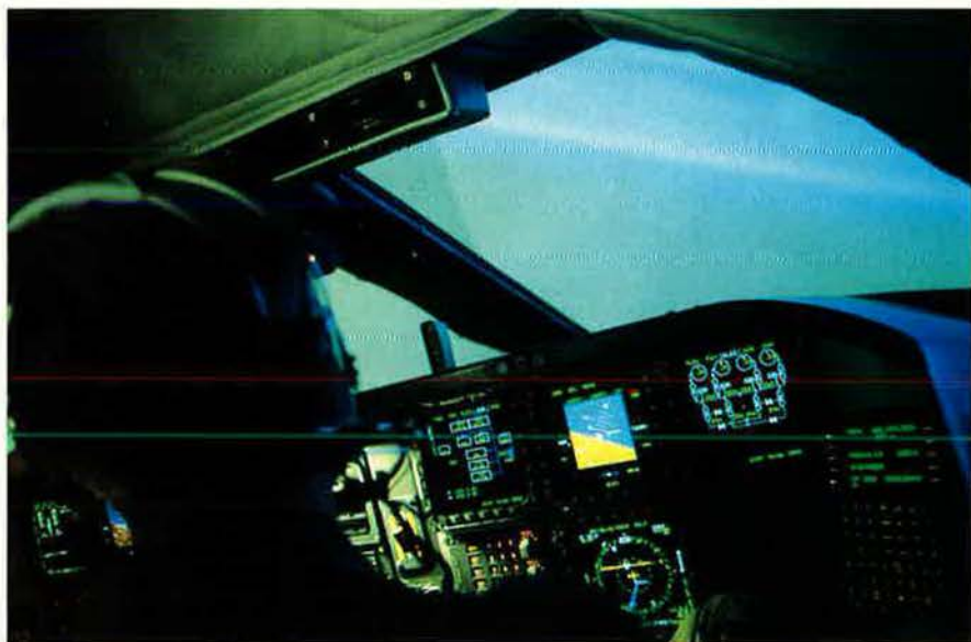
A duplicate of the B-2 cockpit, the Weapon Systems Trainer is used to rehearse training (and, if necessary, combat) missions before pilots fly the real aircraft. Since the full-motion WST runs the same software as the aircraft, maintainers can fix problems on the ground rather than in the air.
