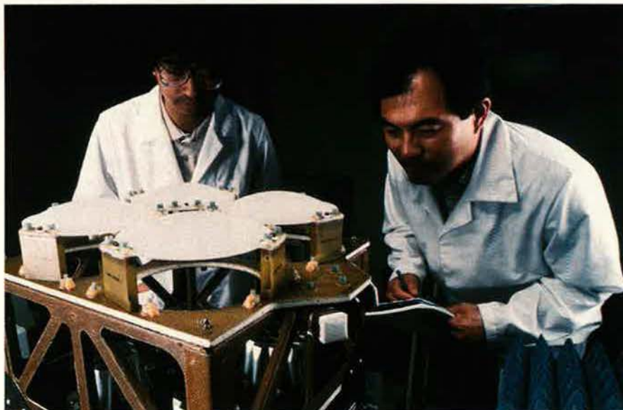
TRW technicians test a Milstar extremely high frequency agile beam antenna at a climate-controlled range. Milstar is a next-generation space communications network designed to relay secure, real-time communications among military users and national command authorities locations worldwide.
