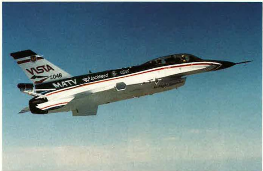
Thrust-vectoring technology provides an alternative method of flight control while increasing the maneuverability of fighter aircraft. The multiaxis thrust-vectoring test aircraft, a modified F-16, proves the technology.
