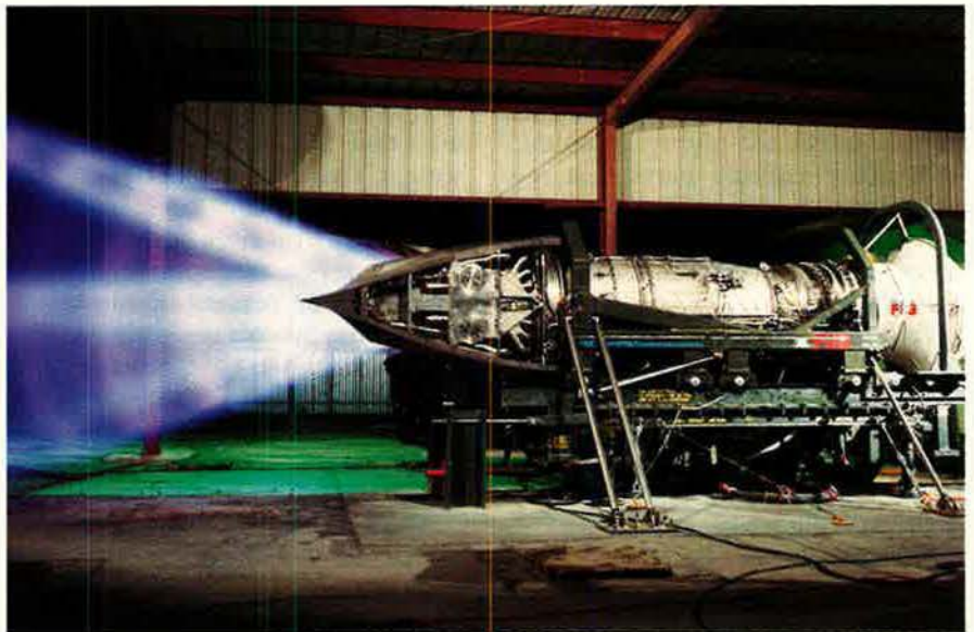
The F-22's Pratt & Whitney F119 thrust-vectoring system helps make the aircraft one of the world's most maneuverable fighters. P&W delivered the first production engine core, above, to USAF in August. The prototype is shown below.
