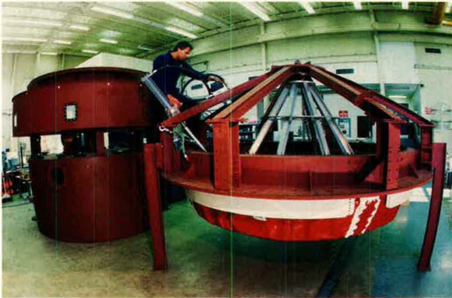
The Air Force will use this Southwest Research Institute equipment to test a heat shield used by the Titan IV Hercules Aerospace Solid Rocket Motor Upgrade program. The test fixture simulates the heat and blast conditions of a rocket launch, from ignition to burnout.
