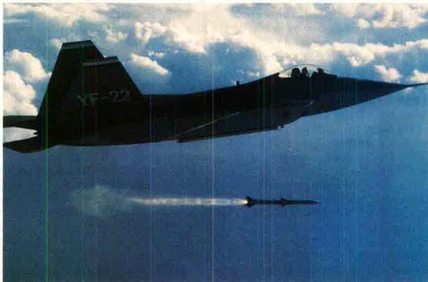
The use of internal weapons carriage, as in the F-22 fighter, allows for a "clean" aircraft, with reduced drag. However, internal carriage also increases the overall weight of the aircraft by ten to fifteen percent.
