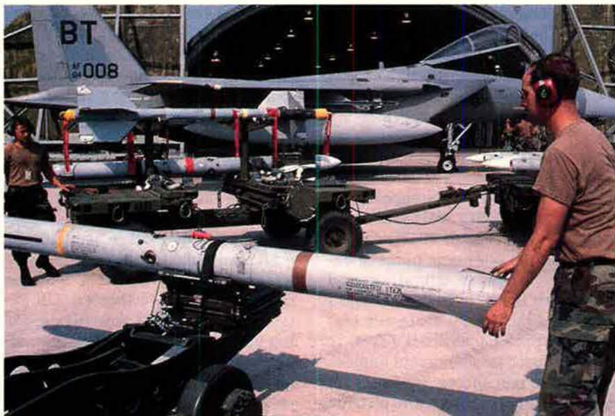
Today's air-to-air weapons, represented by AIM-120s (foreground), AIM-9 Sidewinders, and AIM-7 Sparrows (here with the 36th Fighter Wing at Bitburg AB, Germany), can be improved through modest investment.
