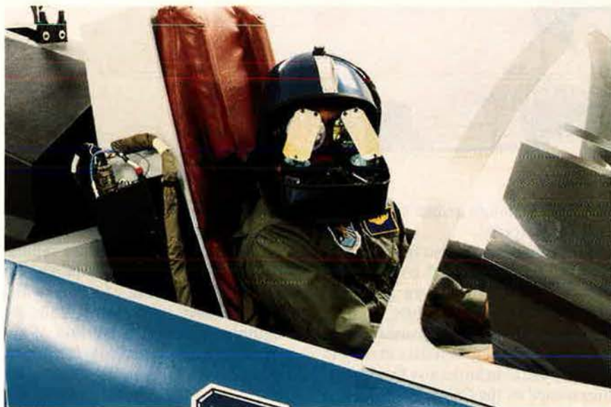
A unique payoff of the Fusion Interfaces for Tactical Environments (FITE) simulator (opposite) is its ability to be configured to present information in a manner of the pilot's choosing. The Air Force is experimenting with a number of different helmet designs in its VCASS program (above).
