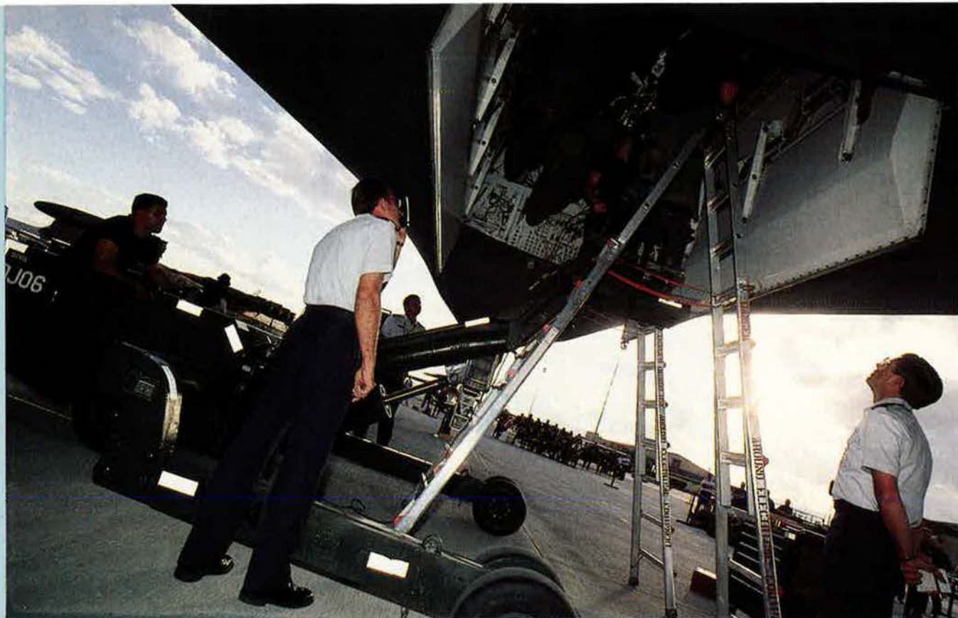
B-1B crews at Gunsmoke were eager to show off their newly acquired conventional capability. Above, during the munitions loading competition, judges observe a crew from the 319th BW loading 500-pound bombs into one of the B-1B's three conventional modules.
