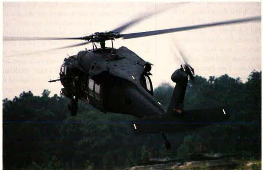
The UH-60 Black Hawk is a workhorse of Army Aviation. Some are equipped for defense (above) with IR gear on the centerline just behind the main rotor engine, heat deflection devices on each engine, and chaff and flare dispensers. The AH-64 Apache (opposite) bristles with high-tech sensors and weaponry for attack.
