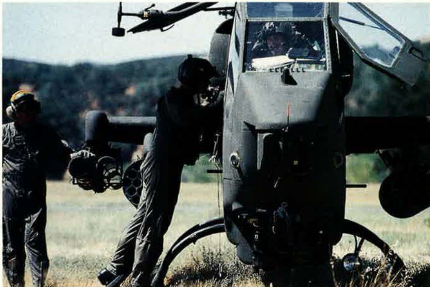
The Vietnam-era Cobra gunship is the Army's most numerous antiarmor-attack helicopter. Its firepower includes a chin-mounted 20-mm or 30-mm gun and eight TOW antiarmor missiles. Below is an AH-1S Cobra from Fort Ord, Calif.
