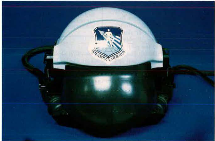
The Air Force has made improvements to this VCASS prototype helmet. Note the size disparity compared to the helmet on p. 32. Future VR helmet systems may not require a transparent visor.
