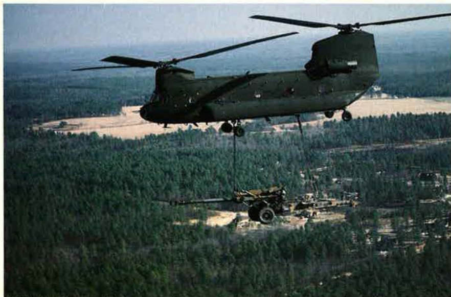
The CH-47D Chinook does a lot of the Army’s lifting. It is the only Army helicopter that can transport a 12.4-ton D5 bulldozer over short distances. Here, a Chinook moves a howitzer and its gun crew and ammunition.
