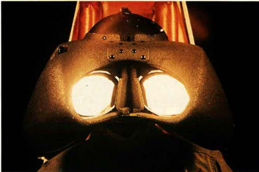
With a look at the old VCASS helmet, it becomes obvious how far the Air Force has come in helmet technologies. Helmet size still must be resolved before virtual reality systems make their way into cockpits.
