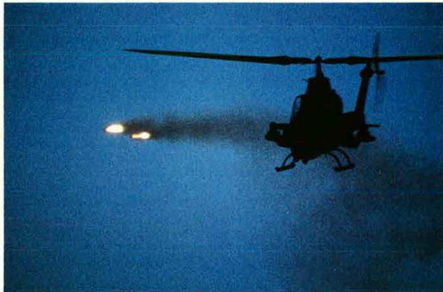
The Vietnam-era Cobra gunship is the Army's most numerous antiarmor-attack helicopter. Its firepower includes a chin-mounted 20-mm or 30-mm gun and eight TOW antiarmor missiles. Below is an AH-1S Cobra from Fort Ord, Calif.
