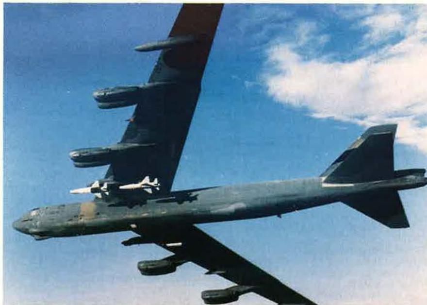
*A B-52 carries AGM-142 Have Nap missiles under its wing. In September flight tests in New Mexico and Utah, the AGM-142, a precision guided, medium-range, conventional standoff missile, demonstrated "superior performance," according to AFMC.*
