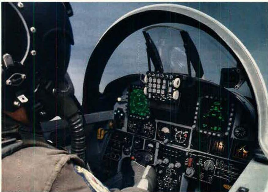
*Northrop's upgraded avionics suite for the F-5, which includes new radar, head-up display, inertial navigation system, and communications and fire-control management systems, is expected to extend the F-5's service life into the next century.*
