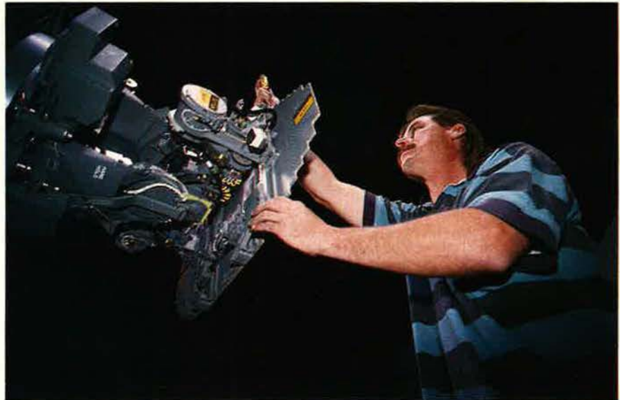
ALCs must continue to prove themselves, says AFMC’s commander, Gen. Ronald W. Yates. Clyde Myers, a technician at Ogden ALC, examines an F-16C/D radar antenna, preparing it for testing.
