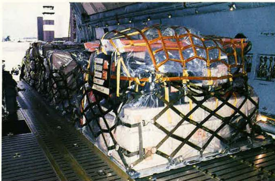
Though the C-5 Galaxy (above) can hold up to 261,000 pounds, its size bars it from many runways around the world. The 363d FW takes its 500,000 pounds of equipment in 12.5 C-141 loads when it deploys.
