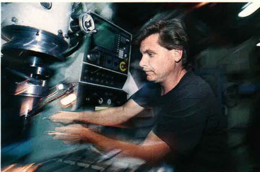
Using a large internal grinder at Ogden ALC, landing gear machinist Dean Tipets grinds the upper bore of a C-141’s main outer cylinder. AFMC operations support all Air Force weapon systems and consume half of USAF’s budget.
