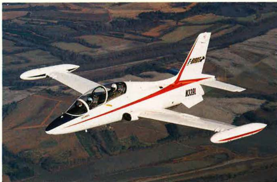
The Lockheed/Aermacchi T-Bird II is the fastest aircraft in the competition, with a top speed of 475 knots. Although it is a high-performance trainer, Lockheed officials say it is a very stable platform.
