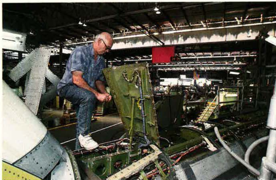
At Ogden ALC, aircraft electrician Lowell Stevens replaces panel fasteners on an F-4's electronics compartment. Careful maintenance is one reason for the long service life of these aircraft.
