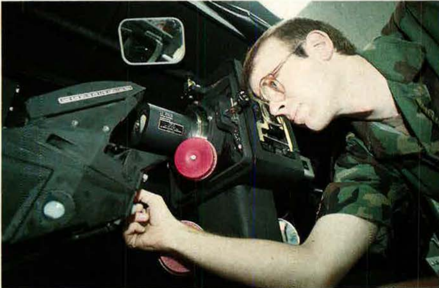
The ten major aircraft programs under Integrated Weapon System Management include the F-16. Above, SSGT. Keith Wolters tests an F-16 head-up display component at Ogden ALC, while co-workers perform F-16 maintenance, below.
