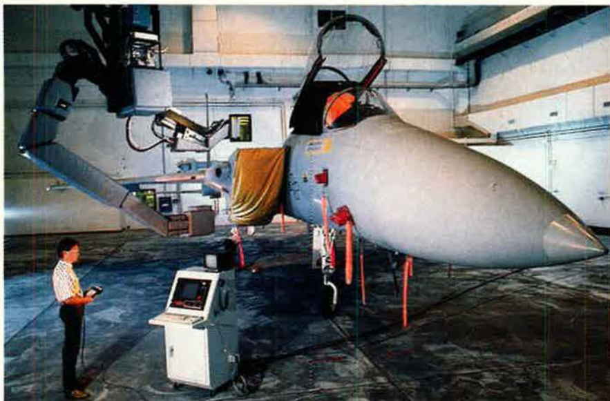
A robotic arm inspects an F-15 (one of the major aircraft programs under IWSM) at Sacramento ALC, McClellan AFB, Calif., scanning the aircraft to detect early signs of cracks and corrosion.
