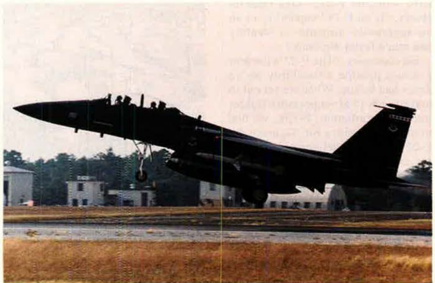
USAF has more than 200 F-15Es, and ACC is pushing for more. The flexible, but decidedly unstealthy, fighter (seen here with AGM-88 HARMs underwing) has been proposed as a successor to the F-4G for the "Wild Weasel" mission.
