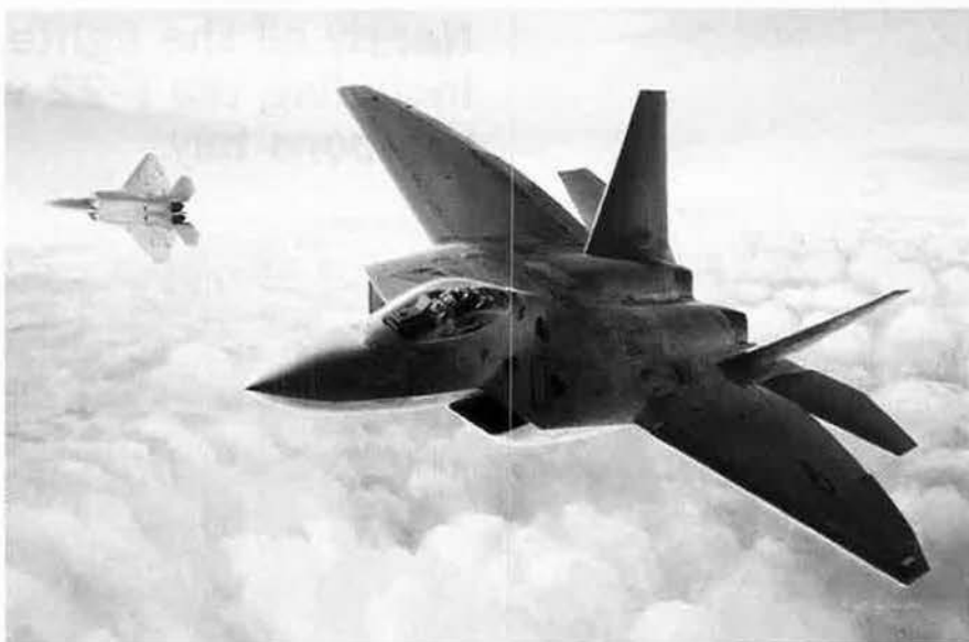
With precision guided munitions carried internally, the F-22 will be a formidable air-to-ground weapon. Requirements chief Maj. Gen. Larry L. Henry praised the fighter's flexibility: "It will be able to do a lot of things."
