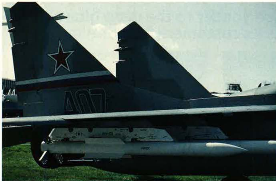
The MiG-29M can carry up to eight R-77s. This new Russian missile, characterized by honeycomb tailfins, is similar to the AIM-120 AMRAAM. Russia plans to include it as standard armament on all late-model aircraft.
