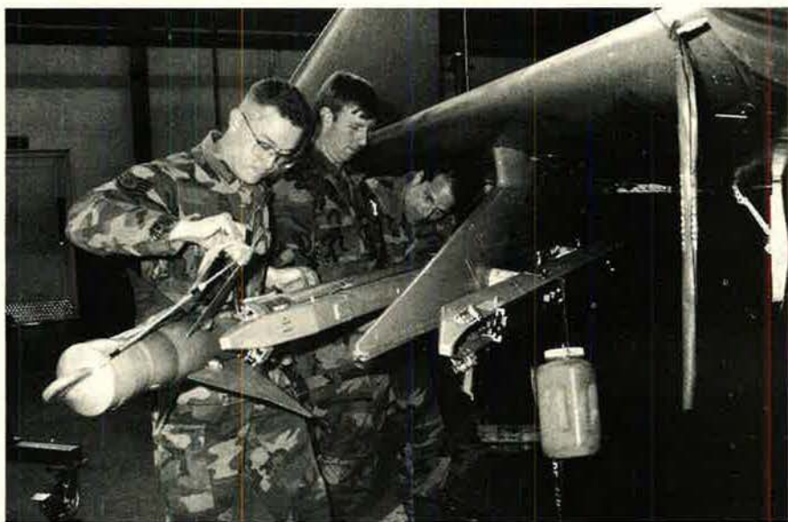
Nevada Air National Guardsmen (from left) MSgt. Steven Privette, TSgt. Mike Muniz, and SMSgt. Mark Frey of the 152d Reconnaissance Group adapt an RF-4C Phantom to carry AIM-9 Sidewinder missiles. The missiles will give the aircraft defense capability for the first time.
