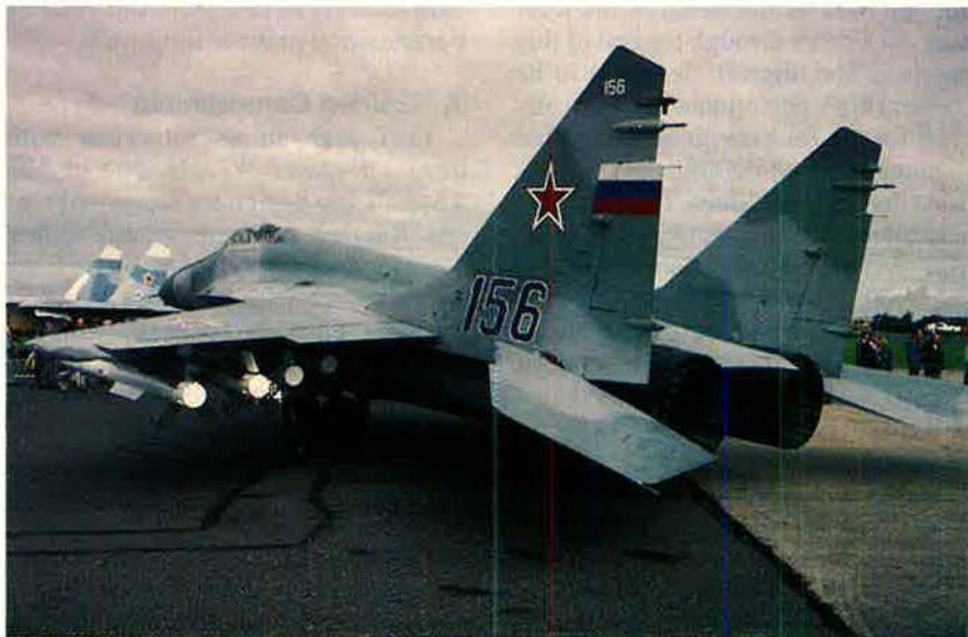
The MiG-29M, a "radical upgrade" of the MiG-29, also debuted at Farnborough in 1992. Aerodynamic modifications to give it relaxed stability make it more maneuverable and more efficient in cruise mode than its predecessor.
