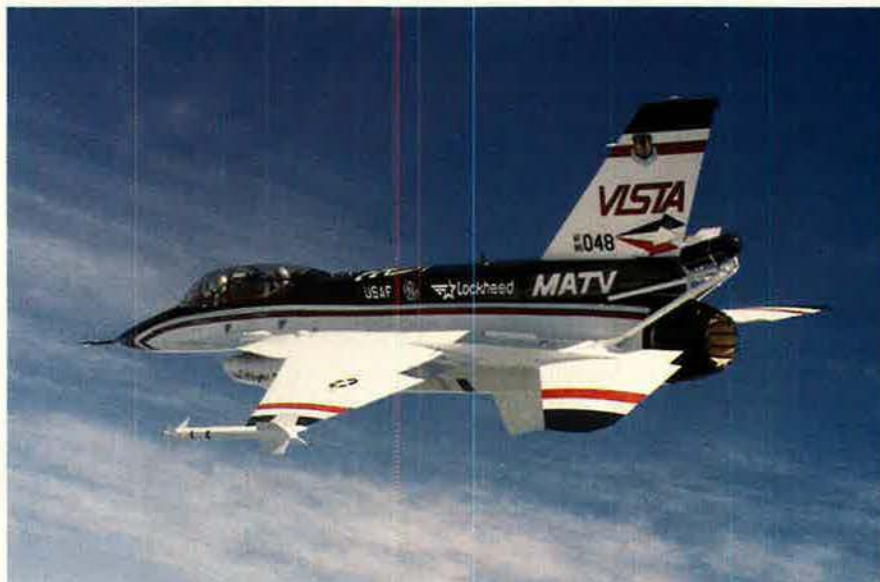
The F-16D Variable Stability In-Flight Simulator Test Aircraft used thrust vectoring for the first time in a July 30 test flight from Edwards AFB, Calif. The aircraft achieved angles of attack of up to 72°, compared to the limit of 25° for the standard F-16. In addition to AOA, yaw and roll rates will be expanded in VISTA/F-16 tests.
