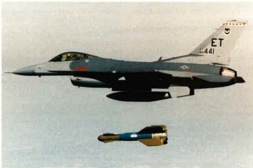
In a demonstration this spring comprising six test flights, an F-16 from Eglin AFB, Fla., delivered precision guided munitions. The tests evaluated technologies for the Joint Direct Attack Munition program. Above, the first PGM, equipped with an Inertial Navigation System/Global Positioning System guidance unit, is released.
