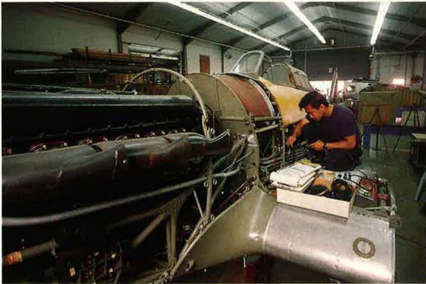
At left, restoration technician Will Lee works on the electrical system of a Hawker Hurricane IIC. The aircraft is about two years from completion. On average, an aircraft requires roughly four years and 50,000–80,000 man-hours to restore. The pace is methodical and meticulously planned. The restoration of an aircraft gives many insights into the construction methods of its time. Interns from various universities go through a ten-week program, gaining valuable knowledge and providing welcome assistance to the full-time staff of thirteen. Below, technician Charlie Parmley applies his expertise to the restoration of Enola Gay.
