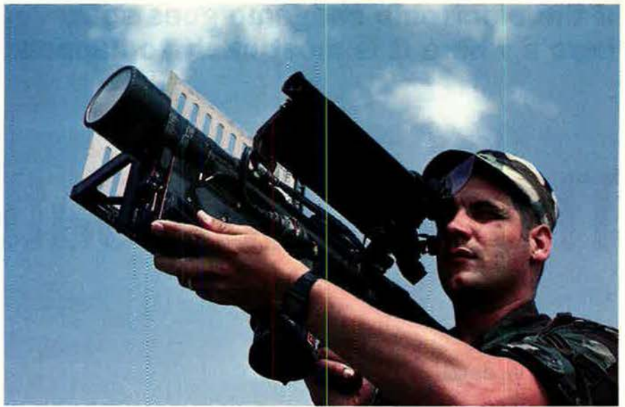
Advanced shoulder-fired heat-seeking SAMs, such as this US-made Stinger, are formidable threats to tactical aircraft and are spreading around the globe. USAF needs new missile approach warning systems to help aircrews thwart SAMs.
