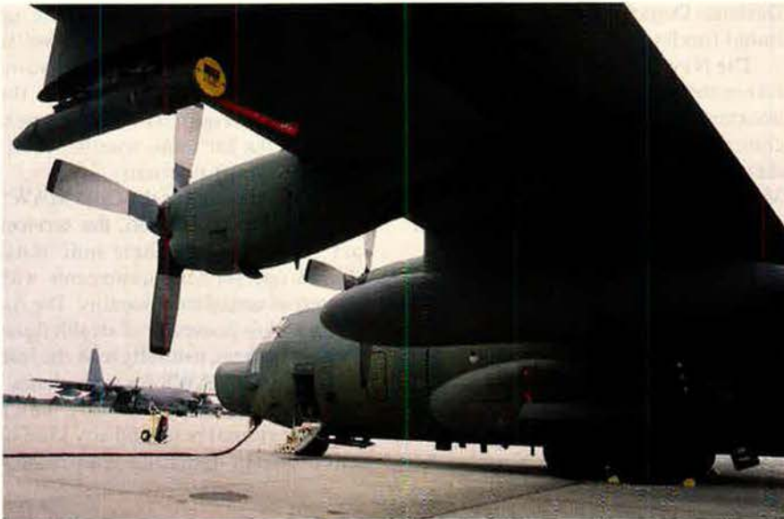
This MC-130H Combat Talon II special operations aircraft comes equipped with the AAR-44 nonemitting passive MAWS to trigger ECMs against radar and IR missiles. Modified airlifter MAWS are slated for fighters.
