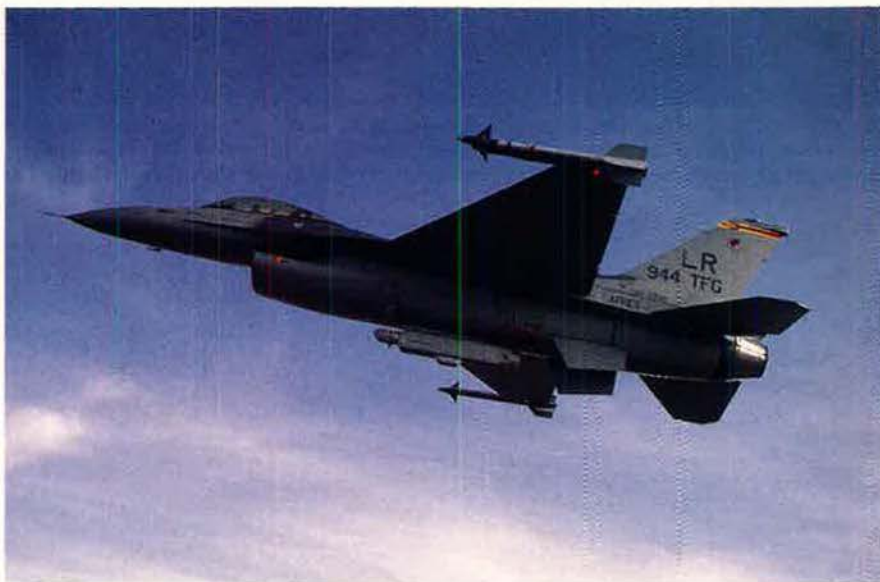
The ALQ-131 radar-jammer pod on the centerline of this F-16C from the 944th Fighter Group (AFRES) at Luke AFB, Ariz., is an example of the electronic countermeasures equipment carried by Air Force fighters and attack aircraft.
