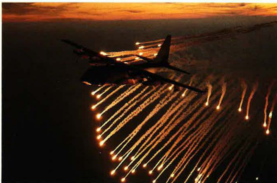
An AC-130 Spectre gunship expends flares in spectacular array to attract incoming infrared-guided missiles and draw them away from the plane. USAF puts a premium on advanced IR countermeasures to protect currently vulnerable planes.
