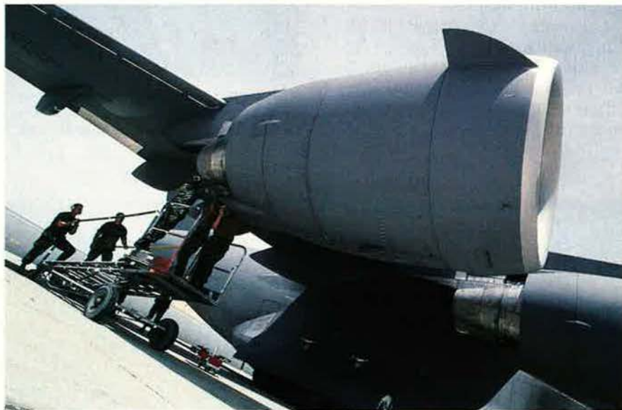
The aircraft's four Pratt & Whitney F117-PW-100 turbofans enable it to carry 160,000 pounds at Mach .77 over distances of up to 2,765 miles. Its short-field landing capability will allow it to operate at airfields as short as 3,000 feet.
