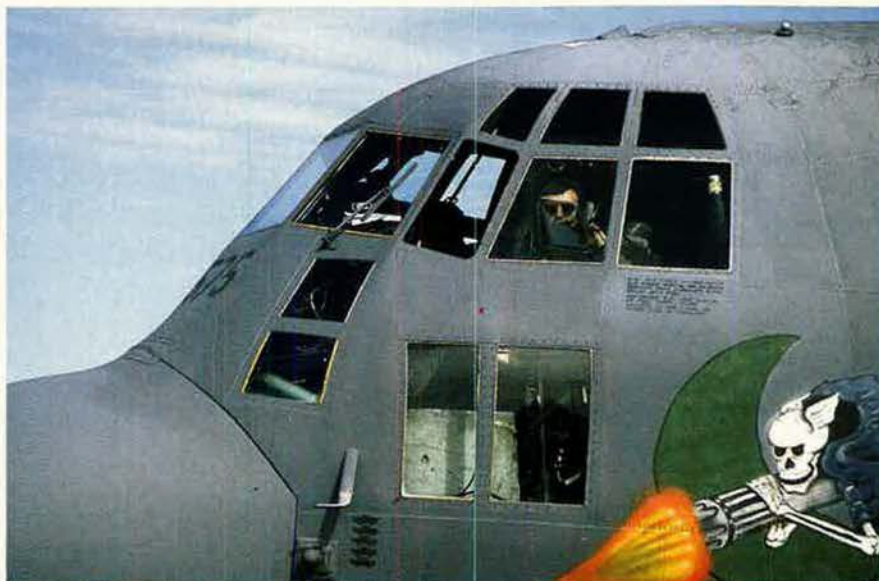
AC-130s often carry colorful and sometimes intimidating nose art. More intimidating are the 40-mm cannon, 105-mm howitzer, and 20-mm cannons it carries. The gunsight of this AC-130 is clearly visible to the left of the pilot's seat.
