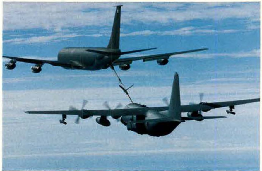
High-performance fighters must slow to the tanker's speed in order to refuel. This AC-130, however, has to accelerate to keep up with the KC-135. With aircraft this large, there is a danger of creating a vacuum between them, causing a collision.
