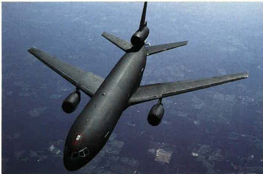
The KC-10 Extender can also double as a transport, making it one of the most versatile airplanes in AMC's inventory. It can refuel both boom and probe-and-drogue aircraft and has a maximum cargo payload of 169,409 pounds.
