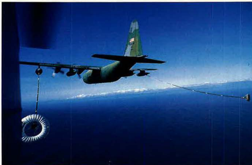
A Marine Corps Reserve RH-53 Sea Stallion chases the "basket" (drogue) of an Air Force HC-130 Combat Shadow from California ANG's 129th Rescue Group. The Combat Shadows do much of their refueling at night.
