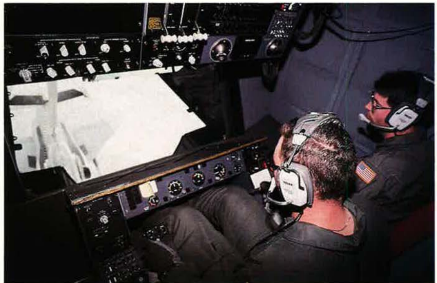
Deployment of the KC-10 marked a great advance in tanker technology. It can carry almost twice as much fuel as the KC-135 and is itself air refuelable. Also, the boom operator's station is pressurized and air-conditioned.
