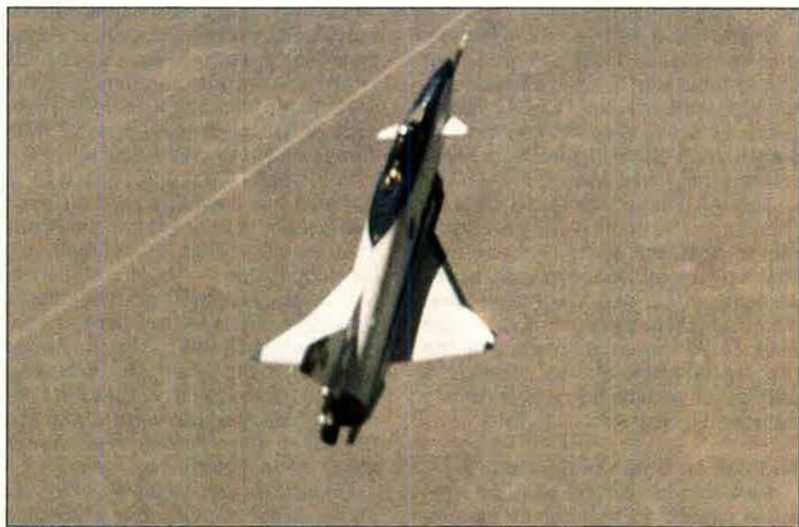
In May, the X-31 Enhanced Fighter Maneuverability aircraft executed a minimum-radius, 180° turn, employing a post-stall technique known as the "Herbst maneuver." Using its full capability of 70° angle of attack, the X-31 can reduce turning time to about two-thirds that of conventional fighters.
