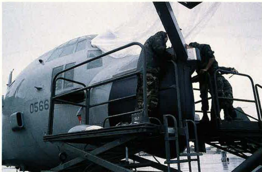
A maintenance crew checks the Fulton Recovery System on an MC-130E Combat Talon aircraft from the 8th SOS. Fourteen MC-130s have been modified with the system, which can pick up loads in midair or from the ground in midflight.
