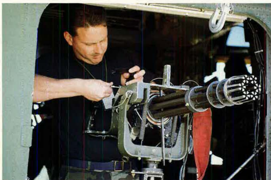
SSgt. Monty Hendrix of the 1st SOW's Weapons Branch fine-tunes a 7.62-mm minigun on a 20th SOS MH-53J Pave Low helicopter. The Pave Low can also carry a .50-caliber machine gun, favored by gunners because of its long range.
