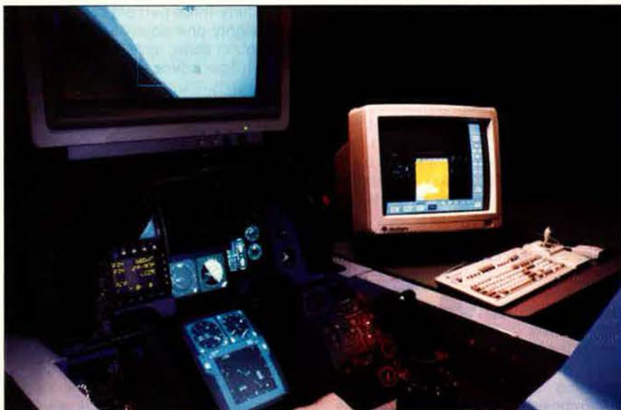
The Air National Guard announced in February the delivery of F-15 and F-16 Part Task Trainers at fourteen Air National Guard squadrons across the US. The trainer is a simulated cockpit device for training in air-to-air, air-to-ground, emergency airstart procedures, and instrument approaches.
