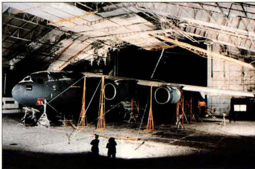
At McKinley Climatic Laboratory, Eglin AFB, Fla., testing of the C-17A has included exposure to temperature extremes of -65° Fahrenheit. In more than 1,550 hours of cold-weather tests, the airlifter's engines idled to provide power for on-board systems, which were then tested for accuracy and reliability.
