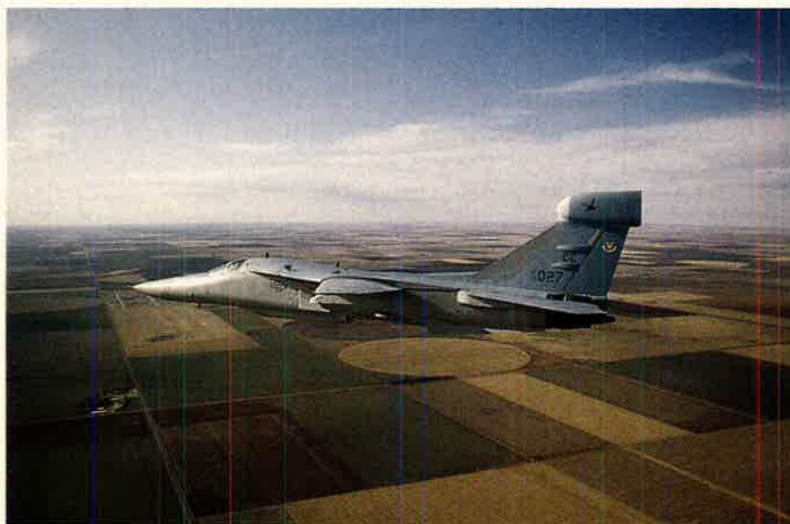
The EF-111A Raven (this one is from the 430th Electronic Combat Squadron, Cannon AFB, N. M.) carries ten jammers internally and can fly with a strike package on the deck, at high speeds, and to extreme ranges.
