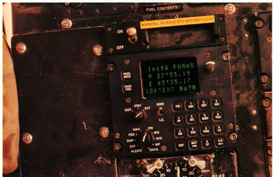
British forces took advantage of the GPS in the Gulf War by equipping Puma helicopters with commercially available GPS receivers. General Horner says GPS is “the wave of the future” and “ought to be in every airplane we fly.”
