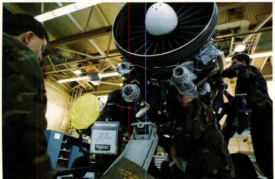
The TF30-P-111, regarded by some as a dinosaur, requires extensive maintenance, but it powers the F-111F to a phenomenal Mach 2.5. Talented Air Force personnel keep the thirty-year-old engines running.
