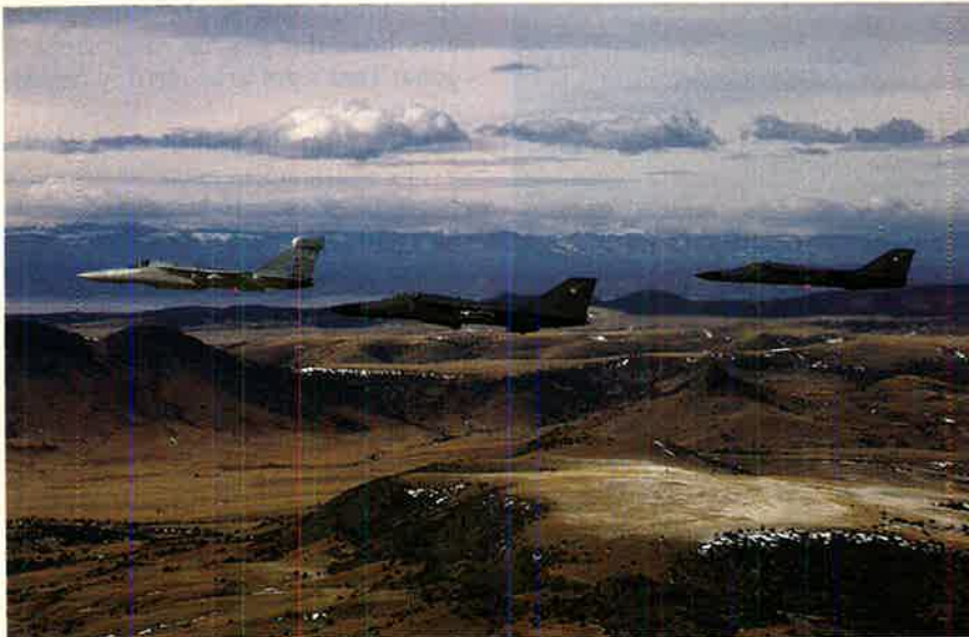
The last of the "Century Series" is represented by an EF-111A (430th ECS), an F-111F (423d FS), and an F-111G (428th FTS). The EF is easily recognized by the pod atop its stabilizer; the F-111F's Pave Tack pod hangs from its weapons bay.
