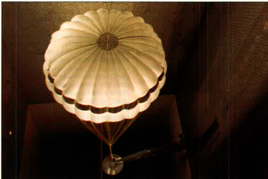
The Huygens space probe is to visit Titan, Saturn's largest moon, in 2002. Parachute deployment and drag performance were verified on a model of the probe (above) in a wind tunnel test at Arnold Engineering Development Center, Arnold AFB, Tenn.
