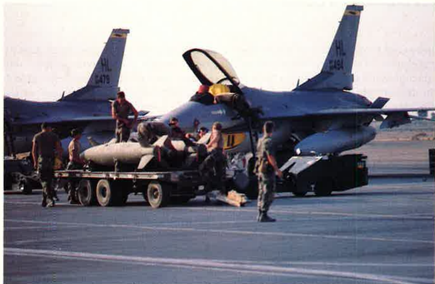
The Killer Scout operation created long days for ground crews. Scouts worked four to six kill boxes at a time. The flight lead usually carried six 500-pound bombs. Other F-16s carried 2,000-pounders (being loaded above).
