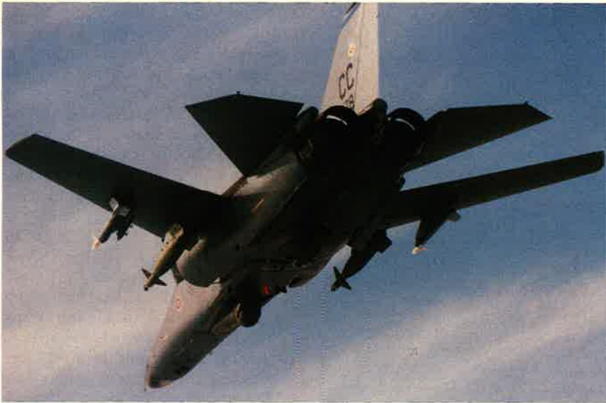
An F-111F from the 423d Fighter Squadron, also at Cannon, shows its stuff in the skies over New Mexico. This Pave Tack-equipped fighter is carrying two 2,000-pound precision guided munitions, an ECM pod, and AIM-9P Sidewinder missiles.
