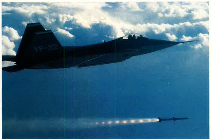
Though it was not required of the prototype, the YF-22 fired an AMRAAM during testing. The F-22 might not carry as many missiles as was originally planned. All will be carried internally to preserve stealthiness.
