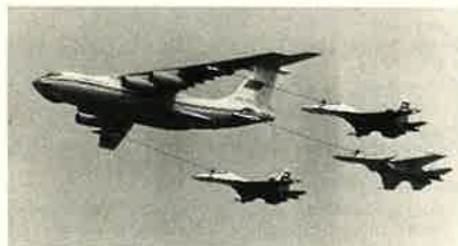
Ilyushin Il-78 ("Midas") refueling two Su-30s and Su-27IB (Piotr Butowski)
