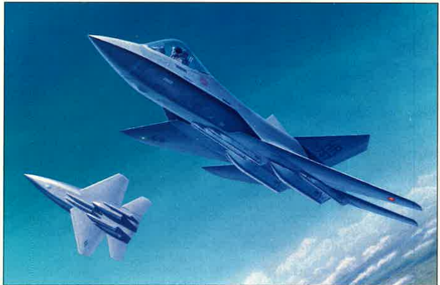
Boeing Defense & Space Group, Military Airplanes Division, is developing a new approach for carrying weapons on existing and future tactical aircraft under a $1.7 million contract with the Armament Directorate of Wright Laboratory, Eglin AFB, Fla. Here, a Multirole Fighter concept is shown with a common weapons carriage system.
