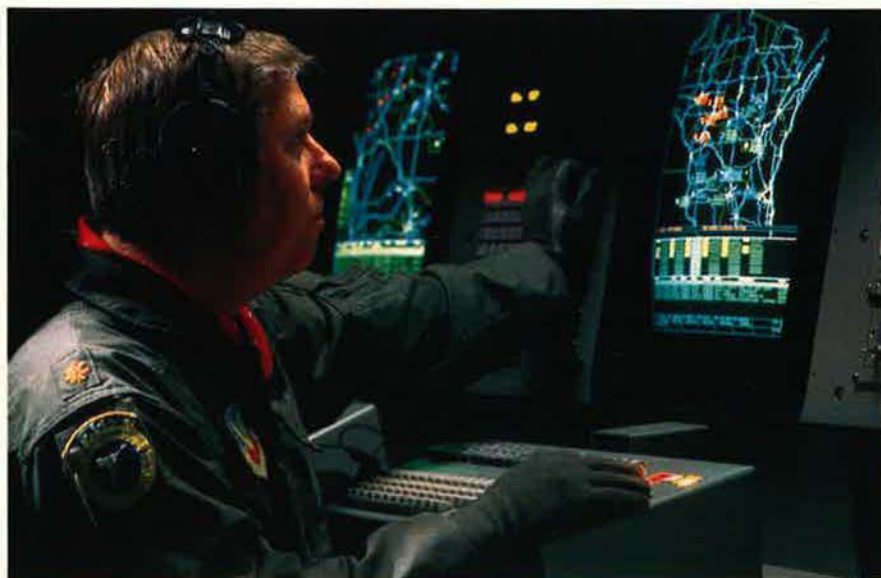
This work station is one of twelve inside an EC-130 ABCCC capsule. ABCCC aircraft worked at night with AWACS and Joint STARS planes in the Gulf War to provide target location updates to inbound fighters and ground commanders.
