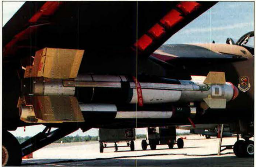
The Rockwell AGM-130 Standoff Weapon System joined the Air Force's missile inventory in November. The system, a powered derivative of the GBU-15, is an air-to-ground weapon for F-111F and F-15E tactical aircraft. It has a low-level stand-off range of fifteen miles and a high-altitude range of forty miles.
