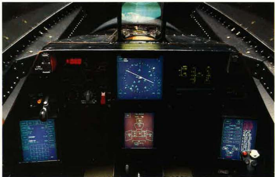
Pilots will reap the benefits of many new cockpit technologies, including larger 3-D tactical situation liquid crystal displays, improved helmets, and data links with other fighters to provide a greater view of the outside world.
