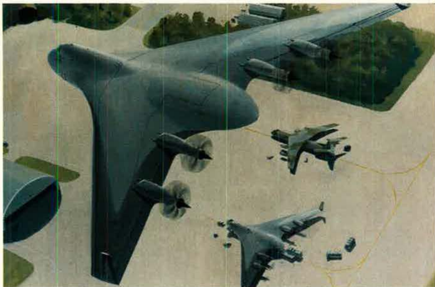
Although the tailless fighter still faces many hurdles, engineers are optimistic about tailless transports (above). The payoffs would be greater fuel efficiency, greater range, and lower observability. The concept has already been proven in the long-range, heavy-lifting B-2.
