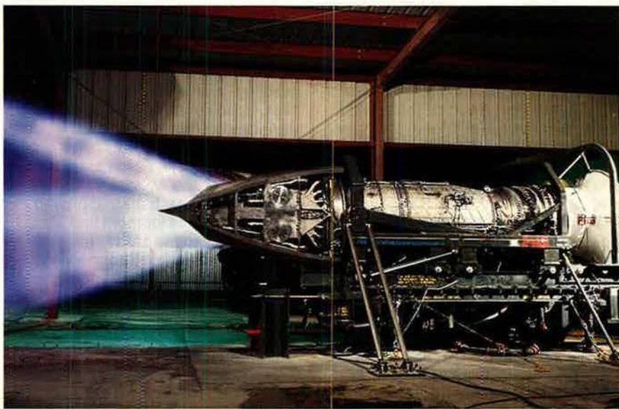
New technologies like those on the supercruising Pratt & Whitney F119 F-22 engine (above) are helping shrink the weight and size of systems while increasing the range, agility, and stealthiness of future aircraft. One concept is the tailless swing-role fighter (opposite).
