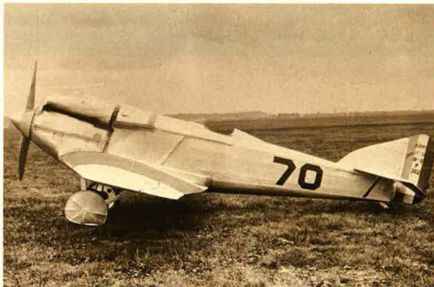
The Verville-Sperry R-3 low-wing monoplane, winner of the 1924 Pulitzer race, inspired Sydney Camm's design for the Hawker Hurricane, but was not developed further by the US Air Service, which continued to fly biplanes until 1934.
