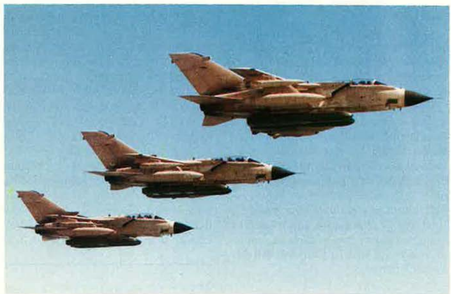
RAF Tornados in desert camouflage carry JP233 systems for low-level runway attacks. In their 1,650 Gulf War combat sorties, GR. Mk. 1s attacked with laser-guided Paveway II weapons, ALARM antiradar missiles, and 1,000-pound bombs.
