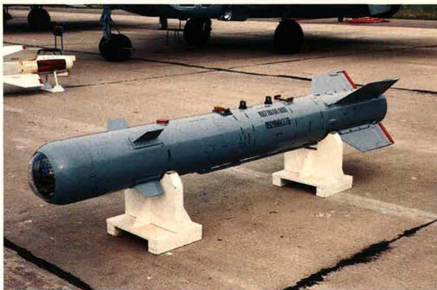
The 1,235-pound KAB-500Kr is a television-guided aerial bomb designed to destroy stationary targets with its 837-pound warhead. Its cousin, the KAB-1500L-Pr, can pierce targets encased in up to seven feet of concrete.
