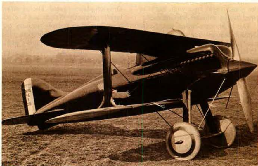
1st Lt. Russell L. Maughan, the 1922 Pulitzer winner, flew this Curtiss R-6. His brush with G-induced loss of consciousness during the race caused widespread alarm among pilots and led to the adoption of safer conditions for later races.
