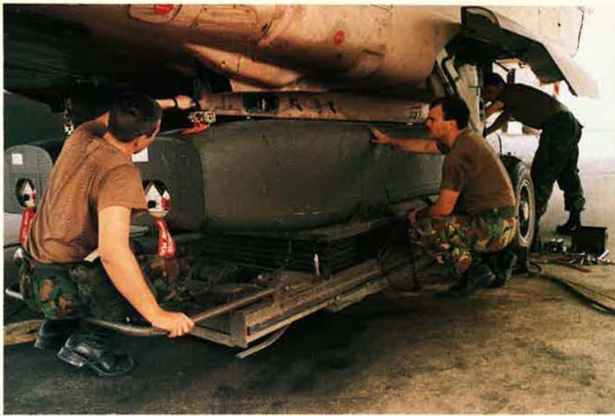
Weapon technicians install the JP233 system on a Tornado. When loaded with a full complement of munitions, each container weighs 5,000 pounds; together the two pack 490 SG357 runway-cratering bomblets and HB876 area-denial mines.
