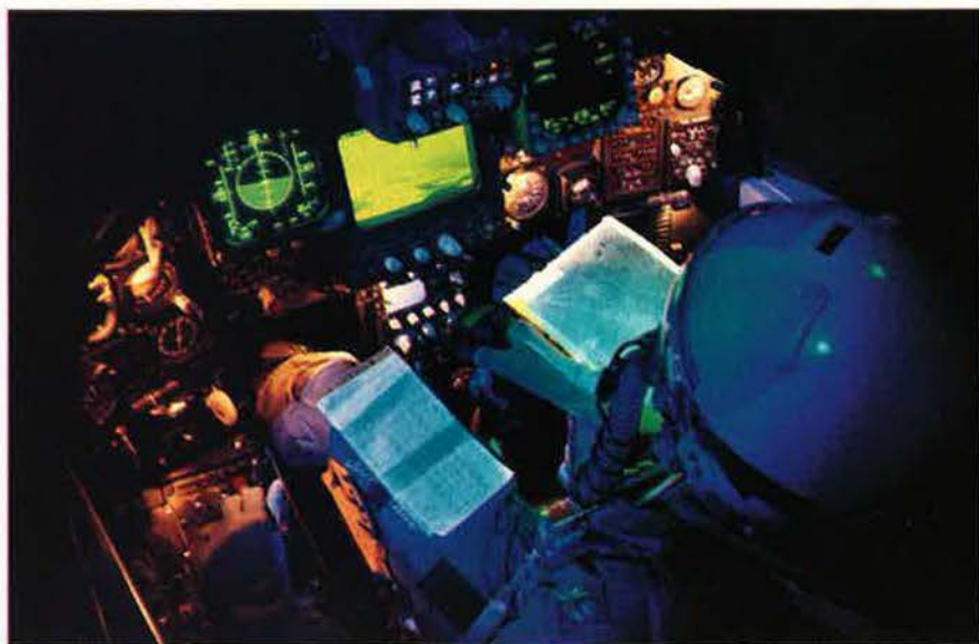
This realistic mission simulator shows the abundance of information at the pilot's disposal, especially from the forward-looking infrared display at center. A new wrinkle has been added: the Pilot Activated Automatic Recovery System.
