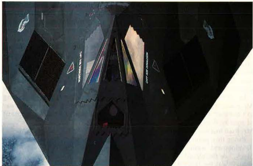
The plane's detractors had a field day mocking the angular surface of the F-117, but the faceting was vital, deflecting radar so that it was impossible to detect the aircraft in time for an enemy to take action.
