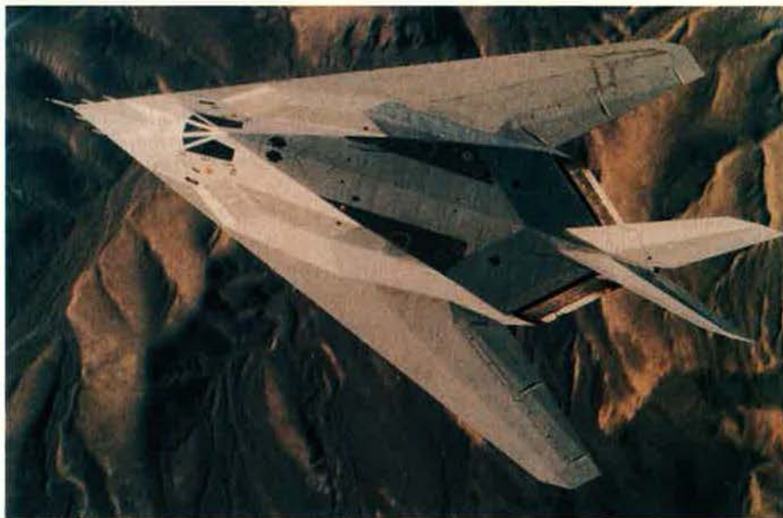
The full-scale development aircraft of the Senior Trend program (above) lacked the F-117's distinctive black coloring, which was strictly an aesthetic choice that had nothing to do with the aircraft's stealthiness.
