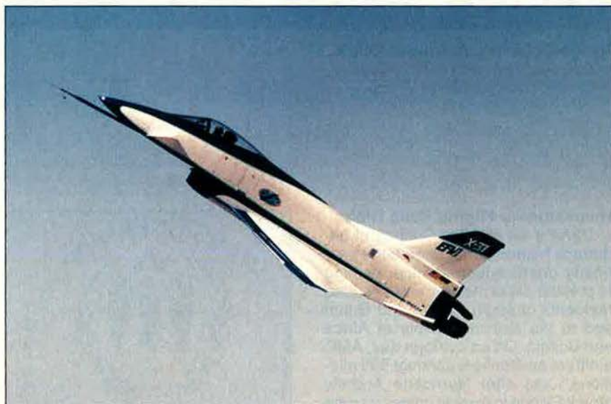
The X-31 first reached an angle of attack of seventy degrees during a research flight at NASA's Ames Dryden Flight Research Facility, Edwards AFB, Calif., in September. The enhanced fighter maneuverability demonstrator uses thrust vectoring and advanced flight control systems to achieve high angles of attack.
