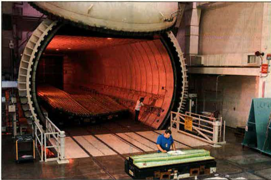
In Seattle, Wash., Boeing Defense and Space Group employees work on B-2 composite components in front of the world's largest autoclave. The two twenty-five-foot by ninety-foot structures are used to cure composite parts for the Stealth bomber with heat and pressure.
