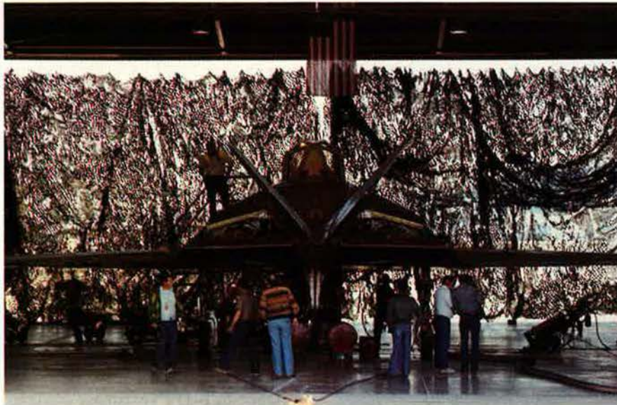
A highly classified system, the F-117 flew only at night for its first five years. Here, technicians work behind camouflage netting. Note exposed engines, normally behind plates to avoid detection of blades and exhaust.
