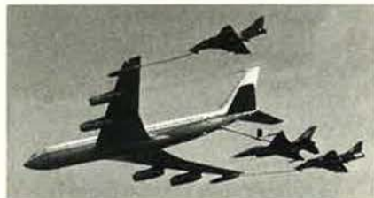
Boeing 707 probe-drogue/flying boom tanker, Israeli Air Force
