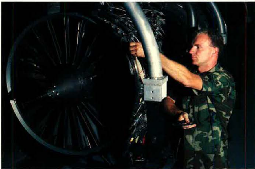
A1C Robert Wilson tends an F100/220 fighter engine in a Mountain Home engine shop. All fighters in the composite wing are powered by variants of the same family of Pratt & Whitney engines. Their commonality is a maintenance boon.
