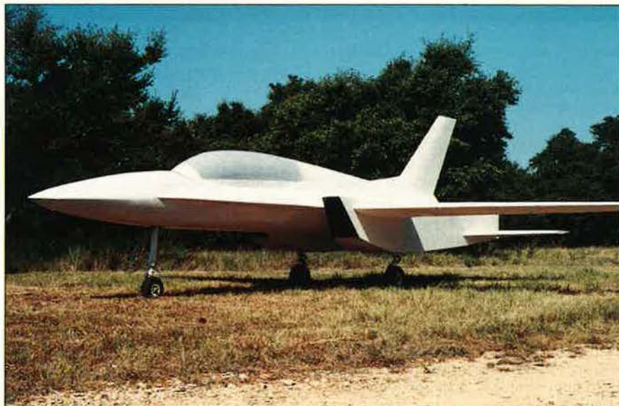
Hamilton Aerospace has completed a ground test of an all-composite prototype aircraft that company President George D. Hamilton plans to propose for the Joint Primary Aircraft Training System (JPATS) program. The aircraft is thirty-three feet, two inches long and ten feet, two inches high. It weighs a mere 5,150 pounds.
