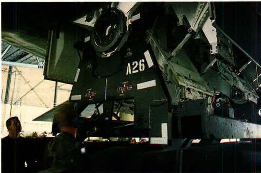
A conventional bomb module is loaded into the B-1 in much the way a toilet paper roll goes into a dispenser. The three modules, which discharge up to twenty-eight 500-pound bombs each, can be clip-loaded or loaded while in the bomb bay.
