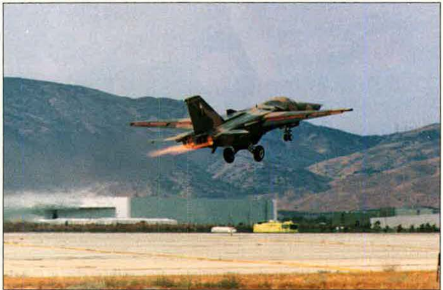
The F-117B Stealth Fighter aircraft took off on July 7, marking the start of functional flight testing in the Pacer Strike upgrade program. Pacer Strike, being carried out by Air Force Materiel Command's Sacramento ALC and Rockwell, should improve reliability and maintainability, navigation, and weapons delivery.
