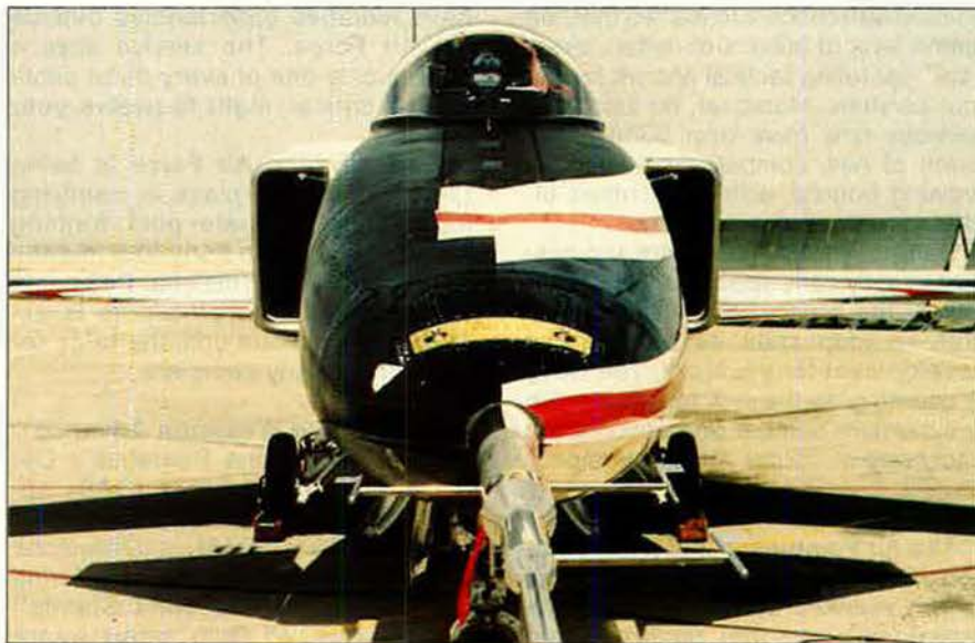
The second X-29 Advanced Technology Demonstrator aircraft was modified with a prototype Vortex Flight Control system. During testing at Edwards AFB, Calif., it proved stable at angles of attack up to fifty degrees. The system includes two slotted nozzles, visible within the lighter area on the nose.
