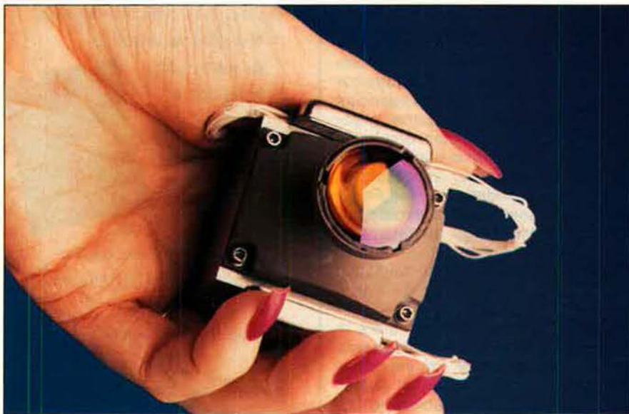
This compact assembly, part of Hughes Aircraft Co.'s Top Hat infrared technology demonstrator, houses a coated optic lens that focuses an observed image on the focal plane array mounted beneath the lens. The system is used to test seekers in a tactical air-to-air environment.
