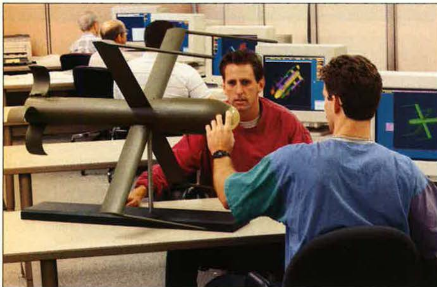
Engineers from Northrop Corp. check the exterior design of the "Bat" prototype. The Bat is a "brilliant" self-guided submunition that autonomously seeks, identifies, and destroys armored moving targets. The Bat is deployed from the triservice standoff attack missile to be used by Air Force and Navy aircraft.
