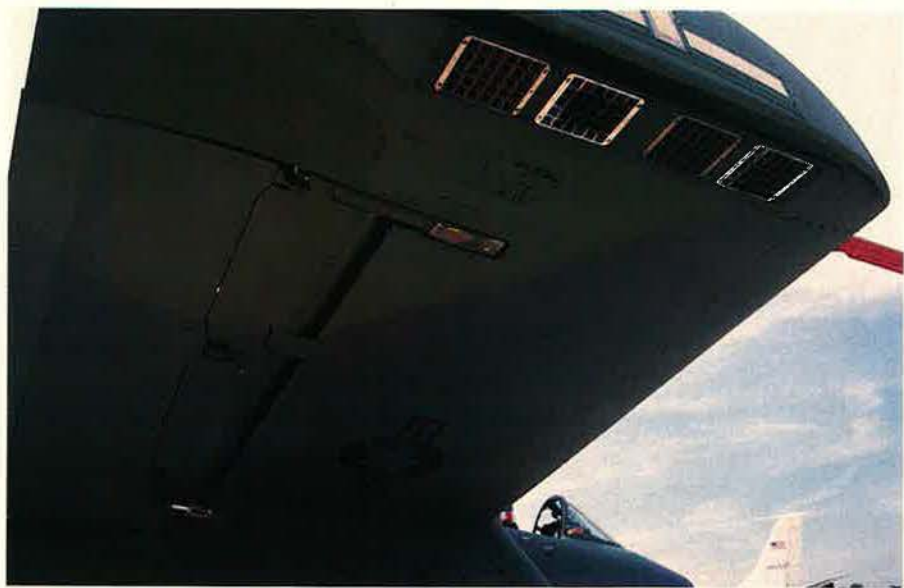
An underwing shot of an A-10 shows one of its four stations for deploying such ECMs as chaff and flare dispensers to counter oncoming radar-guided missiles and infrared-guided, heat-seeking missiles. Flares are becoming more sophisticated.
