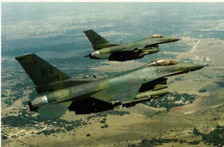
Two F-16 CAS/BAI demonstrators fly a test mission. USAF is studying options to convert 300 Block 30 F-16Cs and Ds to a CAS/BAI variant. The variant would have a night attack system with head-steered infrared and a helmet-mounted display.
