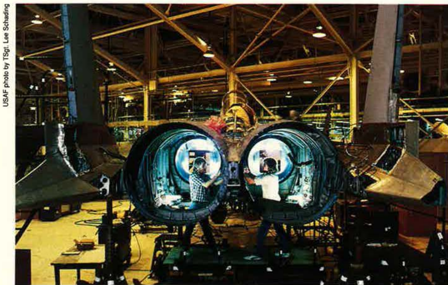
Workers perform multistage improvement program (MSIP) work on an F-15 at Warner Robins Air Logistics Center, Robins AFB, Ga. The MSIP will give 172 F-15A, B, C, and D models new avionics suites.
