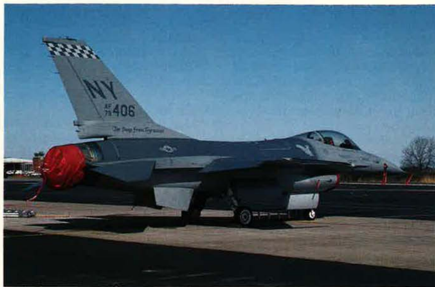
The 174th Fighter Wing of the New York ANG flies F-16As modified with a 30-mm gun pod. Although the unit saw action in Operation Desert Storm, its fighters bear little similarity to what USAF envisions for the Block 30 CAS/BAI F-16s.
