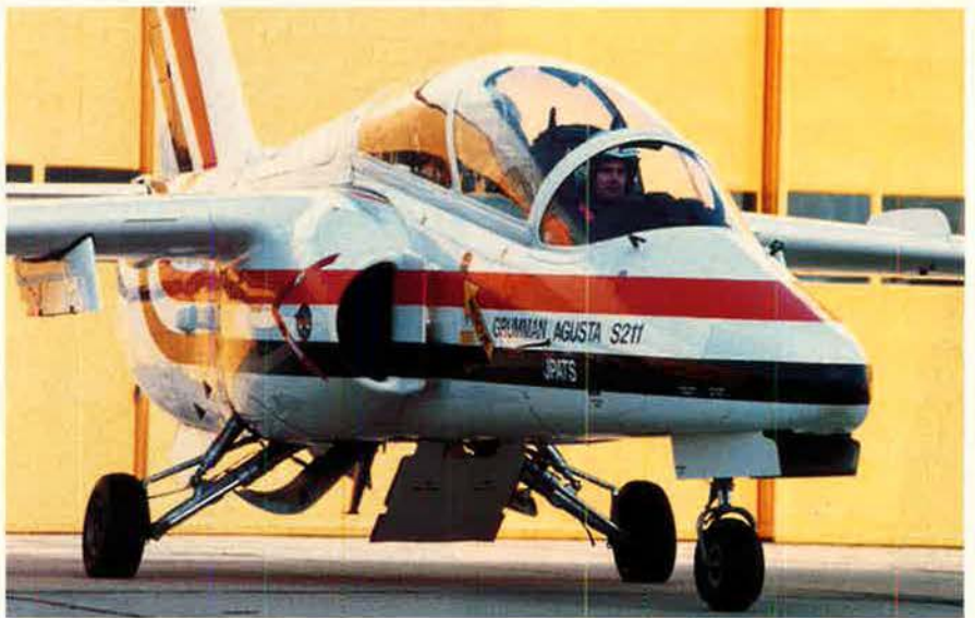
The Grumman/Agusta S211A trainer candidate is powered by the Pratt & Whitney JT15D-5C turbofan engine. Entry-level Air Force and Navy pilots must learn to fly the primary trainer before moving on to greater challenges.
