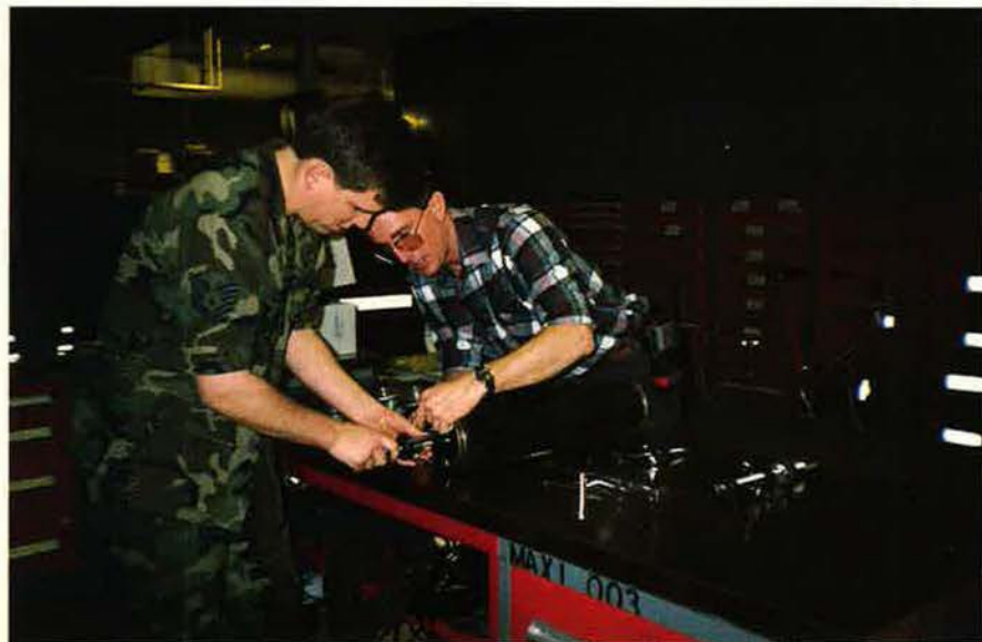
At Travis's C-5 conference, members of the 60th Aircraft Generation Squadron demonstrated a new tool (below) used on commercial airliners to reflare bleed air ducts. The old tool comes in fifty pieces (above, right); the new one (above, left) comes in one piece and adjusts to the size of the duct.
