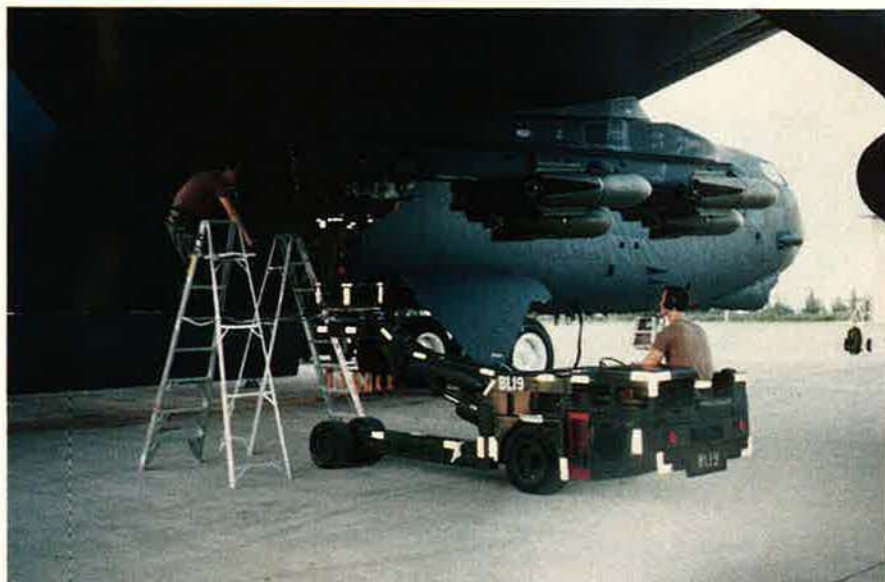
Munitions troops use a "jammer" (a wheeled cart) to lift M117R high-drag iron bombs to the pylon of a B-52, where a technician fastens them in place. These weapons were delivered from low altitude on the second and third nights of the war.
