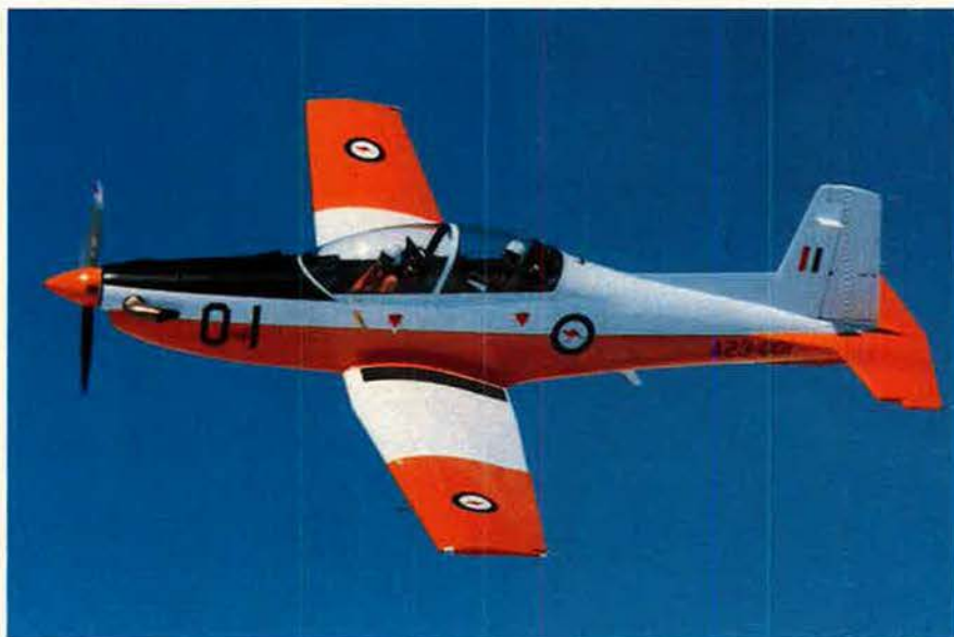
The Beech/Pilatus PC-9 Mk. II, powered by the Pratt & Whitney PT6A-62 turboprop engine, is the only prop-driven aircraft in the competition. The Air Force says it does not matter whether the aircraft is turbofan or turboprop, so long as the aircraft meets requirements.
