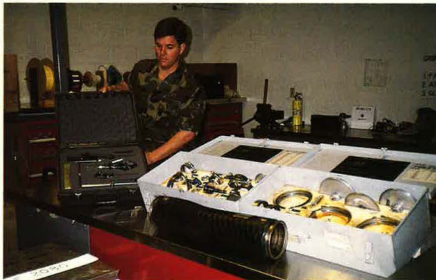
At Travis's C-5 conference, members of the 60th Aircraft Generation Squadron demonstrated a new tool (below) used on commercial airliners to reflare bleed air ducts. The old tool comes in fifty pieces (above, right); the new one (above, left) comes in one piece and adjusts to the size of the duct.
