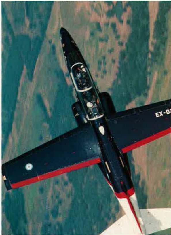
The LTV/FMA Pampa 2000 (a variant of the IA 63) is powered by the Garrett TFE731-2-2B turbofan engine. Both services were seeking a nondevelopmental aircraft to avoid costs associated with developmental programs. Each candidate aircraft fits the bill, according to the Air Force.
