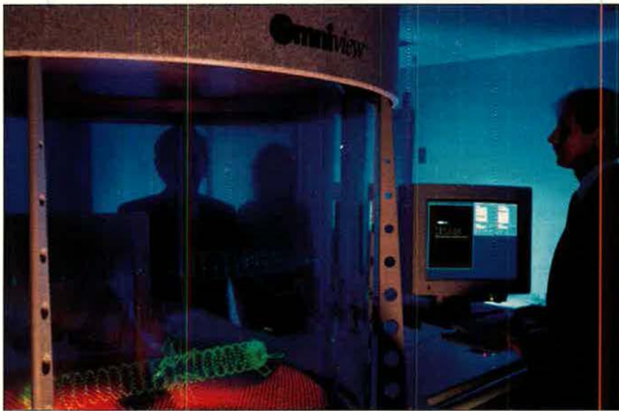
Texas Instruments' OmniView laser-based computer display system produces a true three-dimensional image (here, antitank and antiradar missiles) in real time. The system allows one to view the image from any angle without viewing aids. The image's visual perspective changes with the viewing angle, as with real objects.
