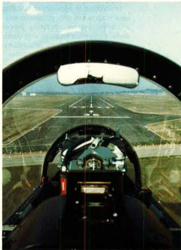
The Lockheed/Aermacchi MB-339 T-Bird II is powered by the Rolls-Royce RB582-01 turbofan. Each aircraft provides stepped tandem seating, as opposed to the T-37's side-by-side seating. At left is the instructor's view from the T-Bird II.
