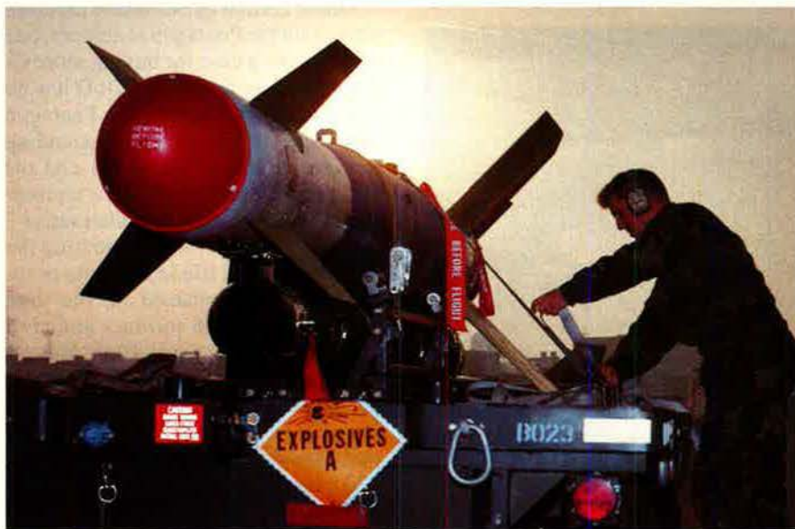
Given multiple demands on its funds, the Air Force can afford to buy only a limited quantity of high-technology standoff weapons such as the AGM-130 (above), a rocket-powered variant of a standard GBU-15 glide bomb. The Air Force also plans to continue development of the Sensor-Fuzed Weapon.
