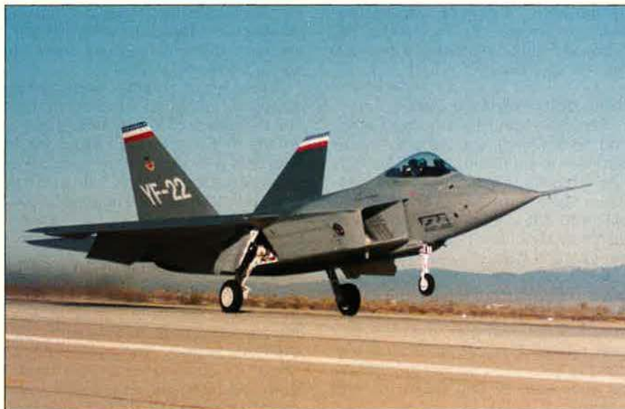
The YF-22 crashed and burned after severe oscillation of the thrust-vectoring nozzles forced it into a gear-up landing. The Air Force said that about ninety percent of the aircraft's testing had been completed. Air Force Chief of Staff Gen. Merrill A. McPeak speculated that an investigation would reveal flight-control software problems.
