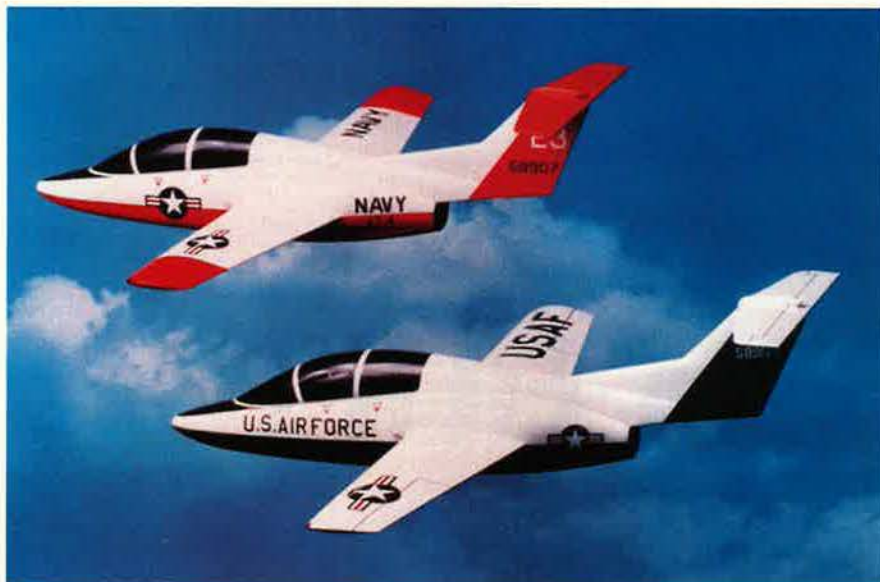
The Rockwell/MBB Fan Ranger (above, models) will use the Pratt & Whitney JT15D-4 turbofan engine. Each proposed JPATS aircraft will require up to twenty percent missionization—the addition of specific technology to enable the aircraft to meet service requirements.
