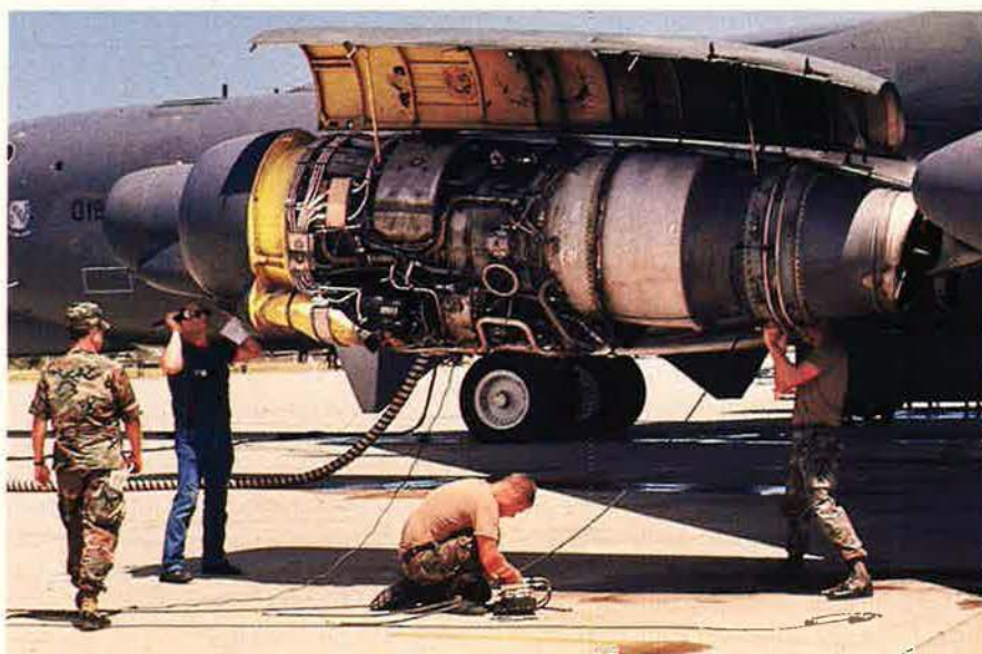
Jet engine mechanics service a thirty-four-year-old J57 engine. Maintenance troops worked fourteen- to sixteen-hour days from the beginning of deployment. The B-52 fleet held an eighty-percent-plus mission capable rate throughout the war.
