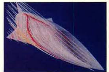
Simulated airflow over a NASP design flying at nearly 17,500 m.p.h.
