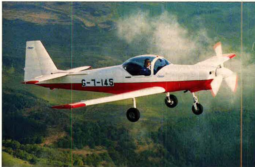
The Air Force chose the team of Slingsby Aviation Ltd. of Great Britain and Northrop Worldwide Aircraft Services, Inc., in late April to build the new Enhanced Flight Screener. The aircraft, a variant of the Slingsby Firefly, will be used to screen prospective pilots for specialized undergraduate pilot training.
