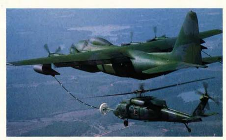
Above, a 9th Special Operations Squadron HC-130 refuels a 55th Special Operations Squadron MH-60 helicopter. Below, a crew loads a howitzer aboard an AC-130 Spectre special operations gunship. AFSOC organizes, trains, and equips all Air Force special operations forces. Its motto is "Air Commandos—Quiet Professionals."
