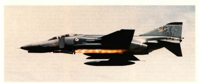
Part of providing a realistic test environment is using equipment already in the inventory to test newer systems. This F-4E is being used to test and evaluate the operational effectiveness of versions of the Maverick missile (here, the AGM-65G). The 2,000 personnel under AFOTEC's operational control form an independent test force with current operational experience.
