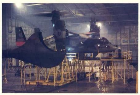
At McKinley Climatic Laboratory, Eglin AFB, Fla., the Bell Boeing V-22 Osprey tiltrotor aircraft is undergoing limited icing, rain, and solar tests. Installation in a raised test fixture allows the aircraft to be run in both helicopter and airplane modes.
