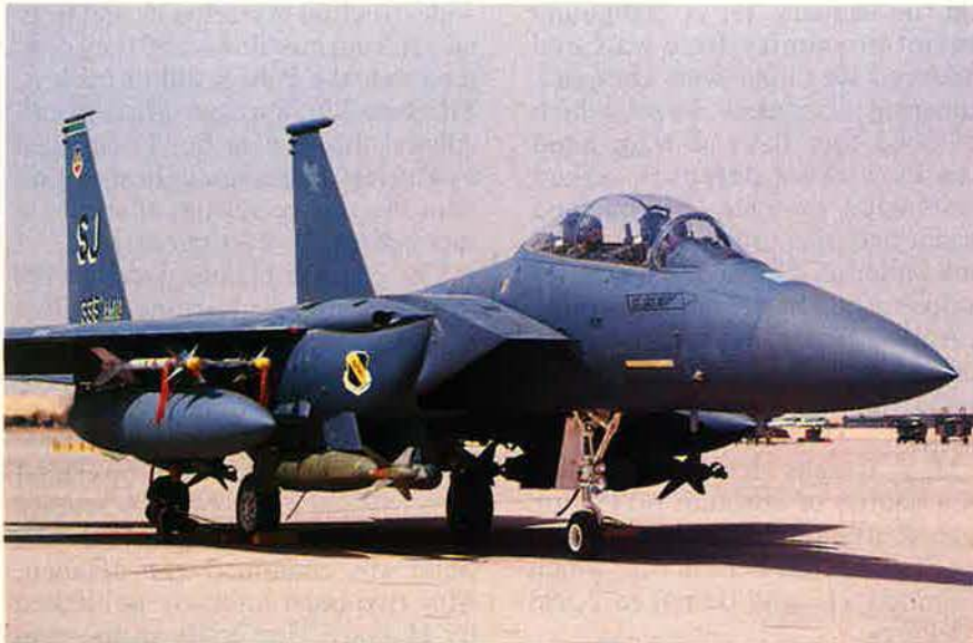
The anti-Scud campaign was not limited to Patriot launches. F-15Es (above, equipped with LANTIRN pods), A-10s, F-16s, and Navy A-6Es joined the hunt. F-14s and S-3s tracked the missiles for the Navy planes, and the F-15Es sometimes got a big assist from the new E-8A Joint STARS aircraft.
