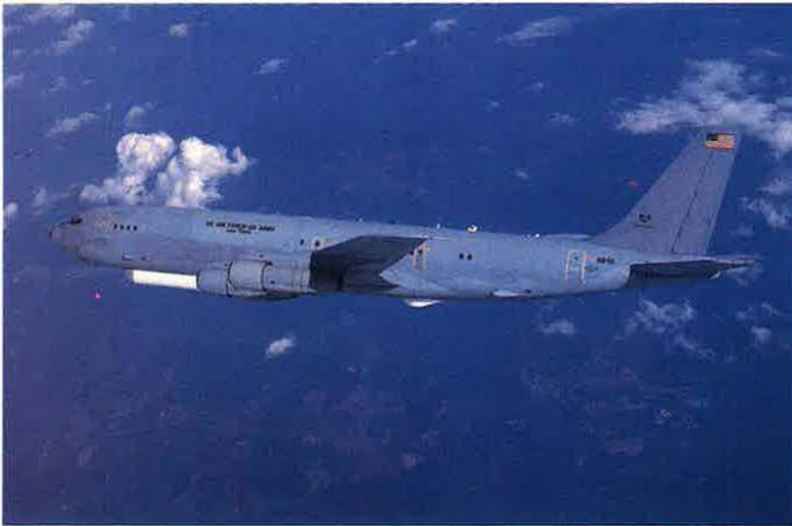
A larger complement of Joint STARS aircraft (only two developmental models were available during the war) will surely help counter future mobile missile threats. Because of the many demands for its data, the modified Boeing 707 with its powerful side-looking radar could only perform Scud-hunting as a sideline.
