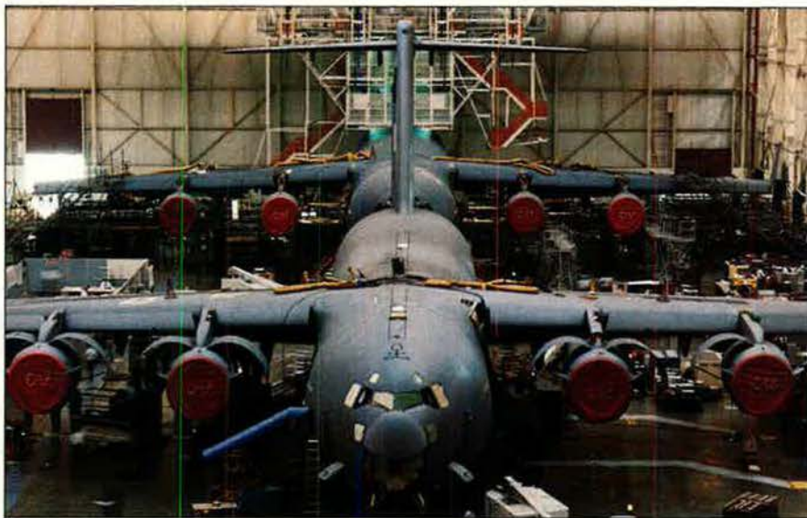
The first two production C-17 airlifters are nearing completion at the McDonnell Douglas Long Beach, Calif., facility. Both are more than ninety percent complete. On-board testing of hydraulic, electrical, and flight-control systems is being conducted before the aircraft are moved to the flight ramp.
