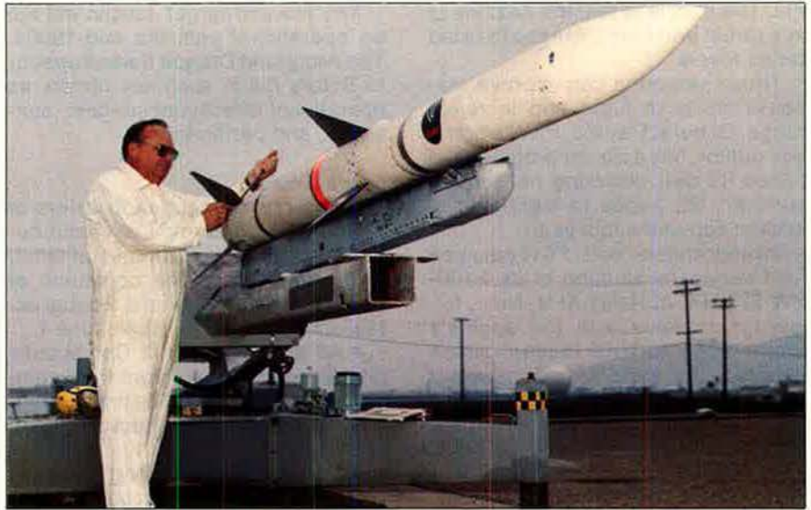
During a February test, this Hughes Advanced Surface-to-Air Missile (ASAM-I) fulfilled its predicted performance parameters. ASAM-I, based on the Advanced Medium-Range Air-to-Air Missile, has a larger rocket motor, designed to provide significantly more impulse and greater range and altitude performance from a ground launch.
