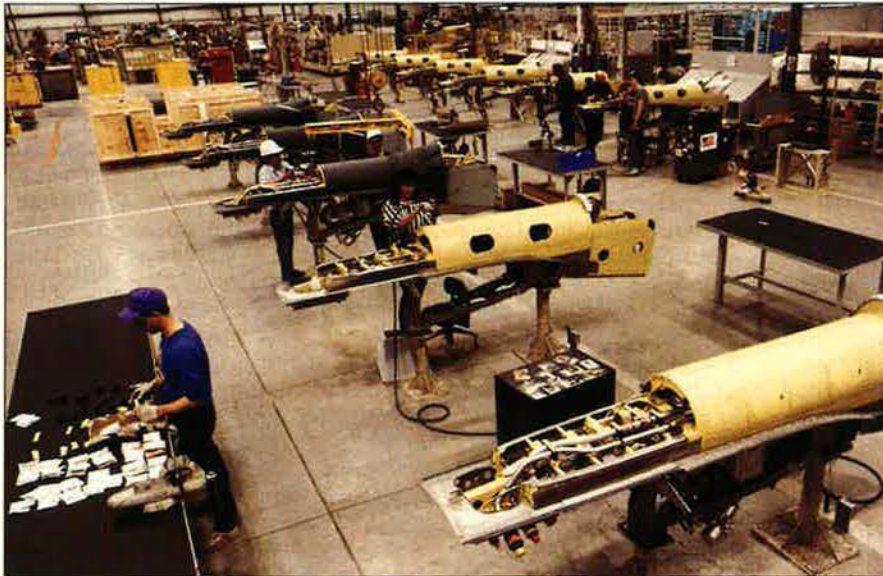
Boeing Product Support Division in Wichita, Kan., has assembled more than sixteen million spare parts to build kits for the KC-135R reengine program since the early 1980s. On February 20, Boeing delivered the 300th kit to the Air Force. Each kit includes struts, nacelles, 12.2 miles of wiring, and other system modification components.
