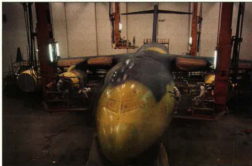
This C-17 P-2 aircraft is having a coat of gray paint applied to its primed surface at McDonnell Douglas's Long Beach, Calif., facility. The P-2, scheduled to be the second production aircraft to come off the assembly line, recently completed fuselage proof-pressure testing and is about eighty percent complete.
