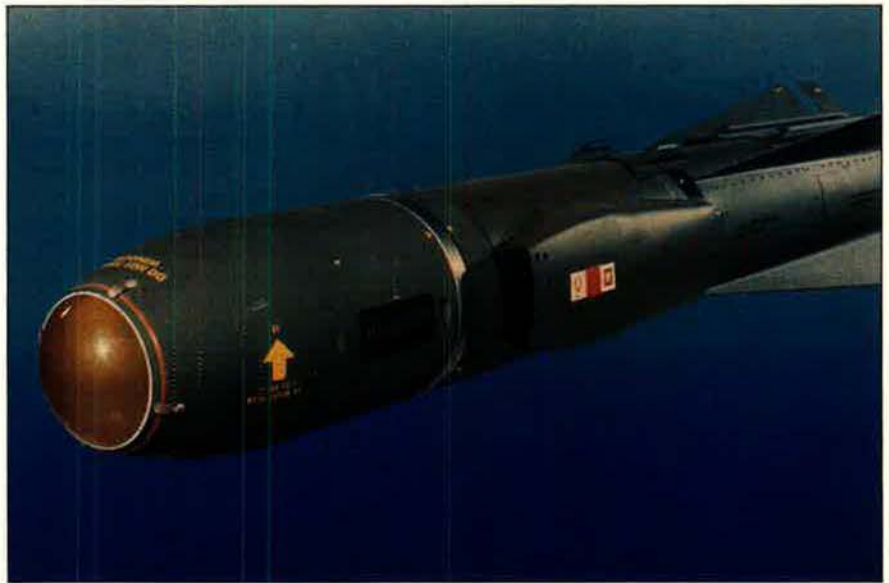
As if Maverick were not effective enough in the Persian Gulf War, Hughes Aircraft Co. has adapted the missile's airframe for an extended-range variant, the Longhorn. A turbine engine designed to travel about forty nautical miles will triple the range of current variants. An infrared seeker or a millimeter-wave radar configuration will allow the new missile to be launched with devastating accuracy.
