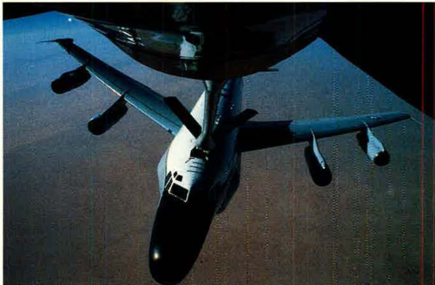
A Rivet Joint aircraft hooks up with a KC-135 for aerial refueling. Such refuelings were enlivened by tanker crew inexperience (which soon wore off), severe weather, and heavy offloads in short durations. Aerial refueling enables RC-135s to remain aloft for extended missions.
